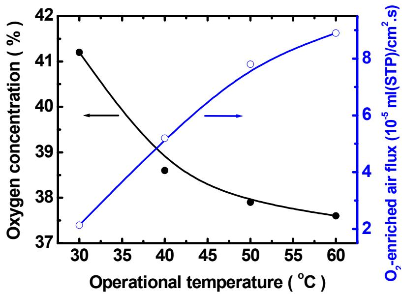
**Fig. S2** Actual air-separation performance through the blend membranes of the MC/AN(30/70) copolymer and 90 wt% ethylcellulose(EC) with operational temperature
