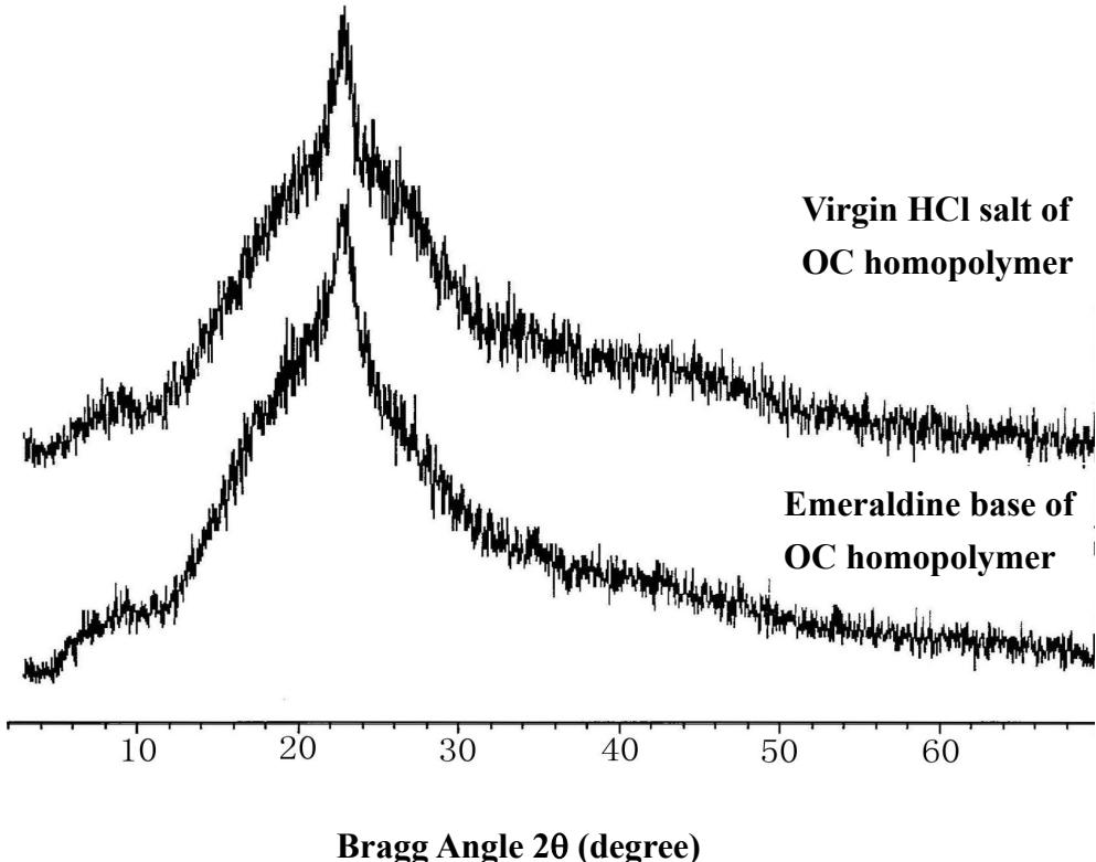
**Fig. S1** Wide-angle X-ray diffractograms of the virgin HCl salt and emeraldine base of OC homopolymer microparticles
