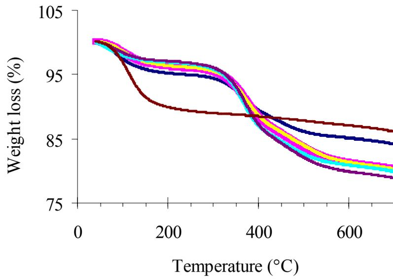
**Figure 2.** TGA graphs of bare laponite (bottom) and laponite that has been reacted with increasing amounts of MPTMS coupling agent.
