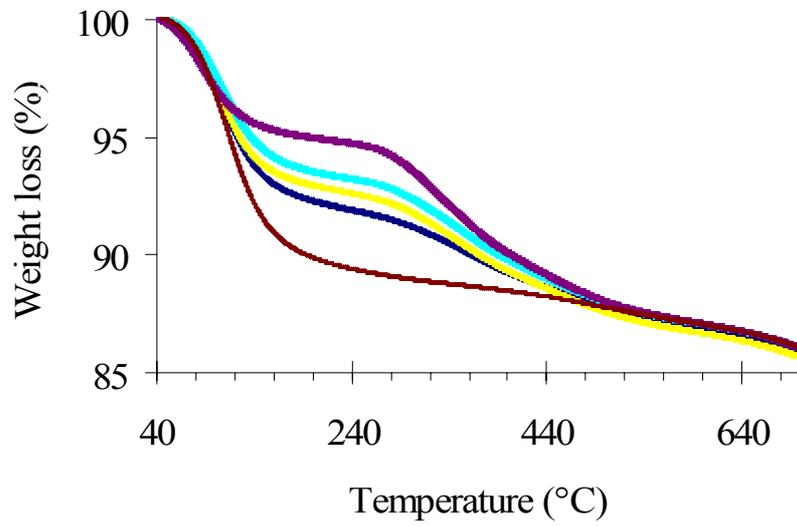
**Figure 3.** TGA graphs of bare laponite (bottom) and laponite that has been reacted with increasing amounts of MPDES coupling agent.
