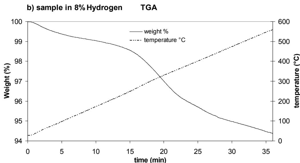
**Fig. 1** TGA of Fe@Au (a) in air; (b) in 8% hydrogen in argon.
