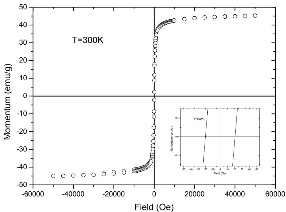
**Fig. 2** Magnetic hysteresis loop at room temperature for Fe@Au core-shell nanoparticles after being washed with 8% hydrochloric acid
