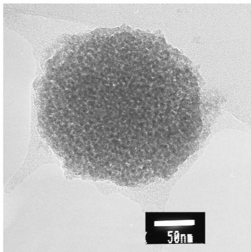
**Fig. 3** Transmission electron microscopy (TEM) image of an “as precipitated” titania nanosphere (*ca.* 200 nm diameter) synthesised *via* controlled hydrolysis of a mixture of novel precursor  $[\text{Ti}(\text{OPr}^i)_3(\text{Krytox})]_n$  and titanium(IV) isopropoxide (TTIP), in supercritical carbon dioxide (Mag. 120 K)
