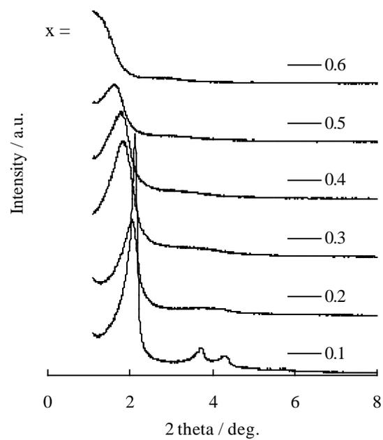
**Figure S1** XRD patterns of surfactant-extracted x-APS-MCM-41, where x is the proportion of APS in the silica sources<sup>20</sup>.
