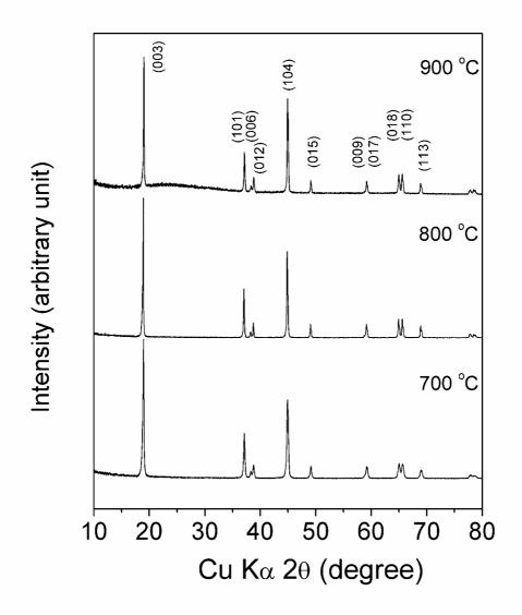
Fig. S3 X-ray diffraction patterns of LiNi<sub>0.5</sub>Co<sub>0.5</sub>O<sub>2</sub> synthesized at various temperatures.
