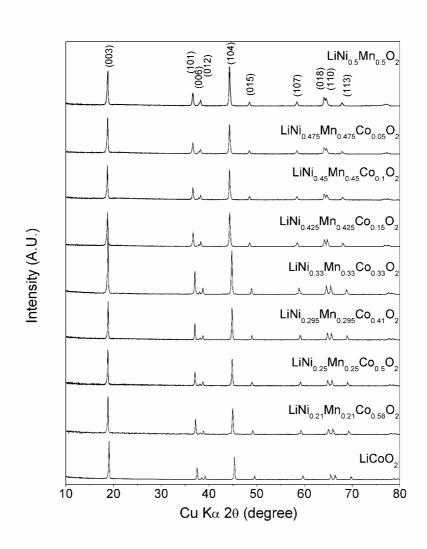
**Fig. S1** X-ray diffraction patterns of  $\text{LiNi}_{0.5-y}\text{Mn}_{0.5-y}\text{Co}_{2y}\text{O}_2$  for  $0 \le 2y \le 1$ .
