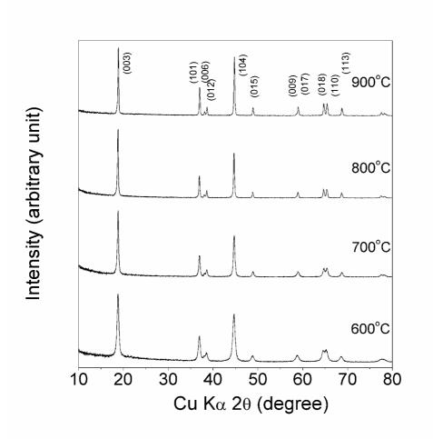
**Fig. S2** X-ray diffraction patterns of LiNi<sub>0.33</sub>Mn<sub>0.33</sub>Co<sub>0.33</sub>O<sub>2</sub> synthesized at various temperatures.
