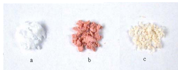
Fig 2. (a) Silica hollow tubes (b) Au-NP silica composite and (c) Ag-NP silica composite samples
