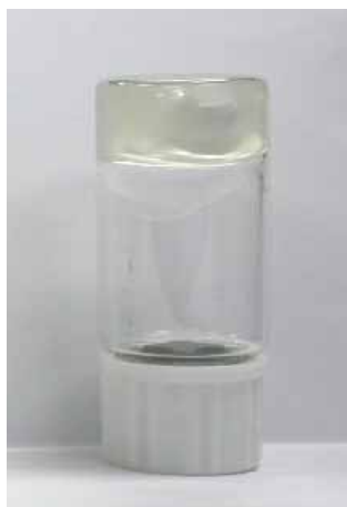
Fig. S4 Photo of BMI·BF 4 -silica (silica: 3 wt% of BMI·BF 4 ) at 20 °C.
