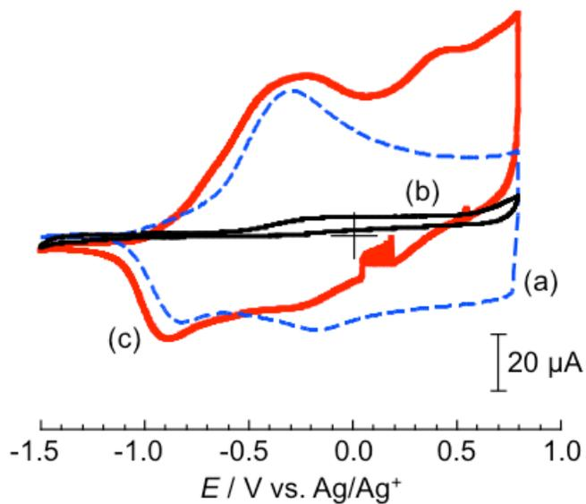
**Figure S3.** (a) CV for a PEDOT film-coated GCE in 0.1 M  $\text{LiClO}_4/\text{AN}$ . Representative CVs for 1 mM 3,4-TBT **2** at (b) bare and (c) PEDOT film-coated GCEs in 0.1 M  $\text{LiClO}_4/\text{AN}$  containing 50 mM  $\text{NH}_4\text{OH}$ . The scan rate in all cases was  $20 \text{ mV s}^{-1}$ .
