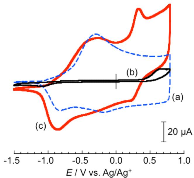
**Figure S8.** (a) CV for a PEDOT film-coated GCE in 0.1 M LiClO<sub>4</sub>/AN. Representative CVs for 1 mM bromo-TBT **8** at (b) bare and (c) PEDOT film-coated GCEs in 0.1 M LiClO<sub>4</sub>/AN containing 50 mM NH<sub>4</sub>OH. The scan rate in all cases was 20 mV s<sup>-1</sup>.
