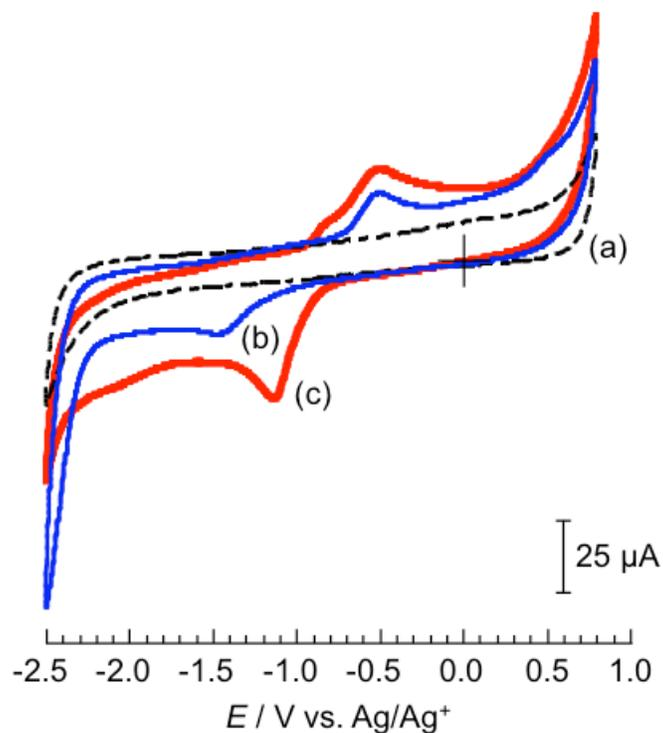
**Figure S2.** (a) CV for 50 mM  $\text{NH}_4\text{OH}$  at a bare GCE in 0.1 M  $\text{LiClO}_4/\text{AN}$ . CVs for 1 mM (b) TT **10** and (c) TBT **1** at bare GCEs in 0.1 M  $\text{LiClO}_4/\text{AN}$  containing 50 mM  $\text{NH}_4\text{OH}$ . The scan rate in all cases was  $20 \text{ mV s}^{-1}$ .
