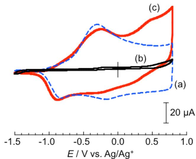
**Figure S5.** (a) CV for a PEDOT film-coated GCE in 0.1 M LiClO<sub>4</sub>/AN. Representative CVs for 1 mM 2,5-dimethyl-TBT **5** at (b) bare and (c) PEDOT film-coated GCEs in 0.1 M LiClO<sub>4</sub>/AN containing 50 mM NH<sub>4</sub>OH. The scan rate in all cases was 20 mV s<sup>-1</sup>.
