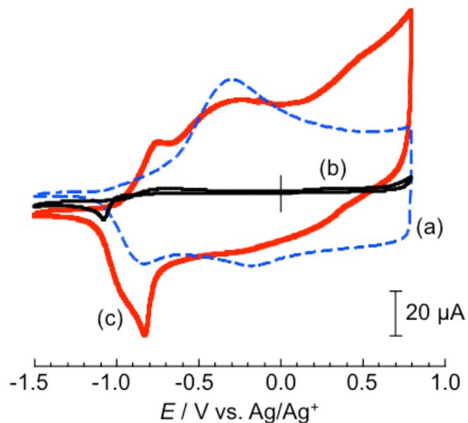
**Figure S4.** (a) CV for a PEDOT film-coated GCE in 0.1 M LiClO<sub>4</sub>/AN. Representative CVs for 1 mM 3,4-dimethyl-TBT **4** at (b) bare and (c) PEDOT film-coated GCEs in 0.1 M LiClO<sub>4</sub>/AN containing 50 mM NH<sub>4</sub>OH. The scan rate in all cases was 20 mV s<sup>-1</sup>.
