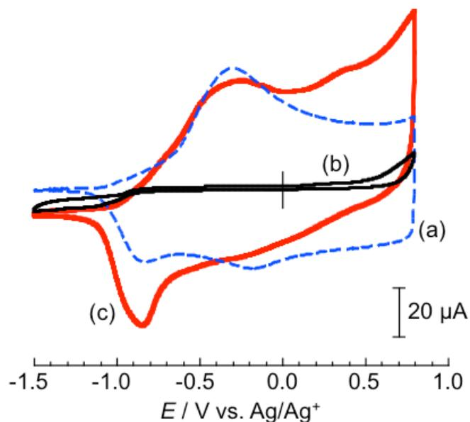
**Figure S6.** (a) CV for a PEDOT film-coated GCE in 0.1 M LiClO<sub>4</sub>/AN. Representative CVs for 1 mM methoxy-TBT **6** at (b) bare and (c) PEDOT film-coated GCEs in 0.1 M LiClO<sub>4</sub>/AN containing 50 mM NH<sub>4</sub>OH. The scan rate in all cases was 20 mV s<sup>-1</sup>.
