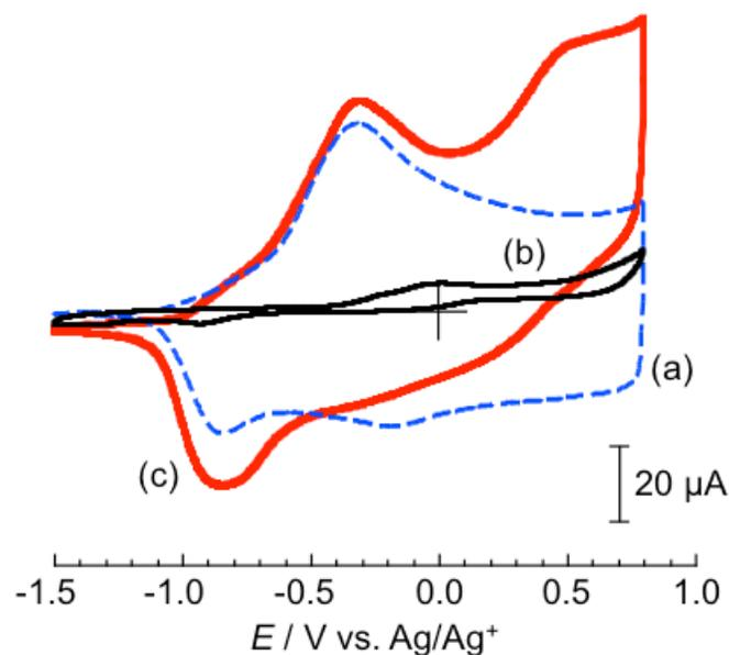
**Figure S7.** (a) CV for a PEDOT film-coated GCE in 0.1 M LiClO<sub>4</sub>/AN. Representative CVs for 1 mM acetyl-TBT **7** at (b) bare and (c) PEDOT film-coated GCEs in 0.1 M LiClO<sub>4</sub>/AN containing 50 mM NH<sub>4</sub>OH. The scan rate in all cases was 20 mV s<sup>-1</sup>.
