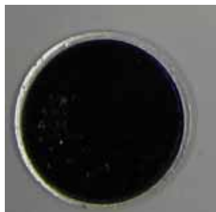
S2 Photograph of an aluminium/alumina disc with tree-like pores after electrodeposition of gold, showing uniformity of gold infiltration.
