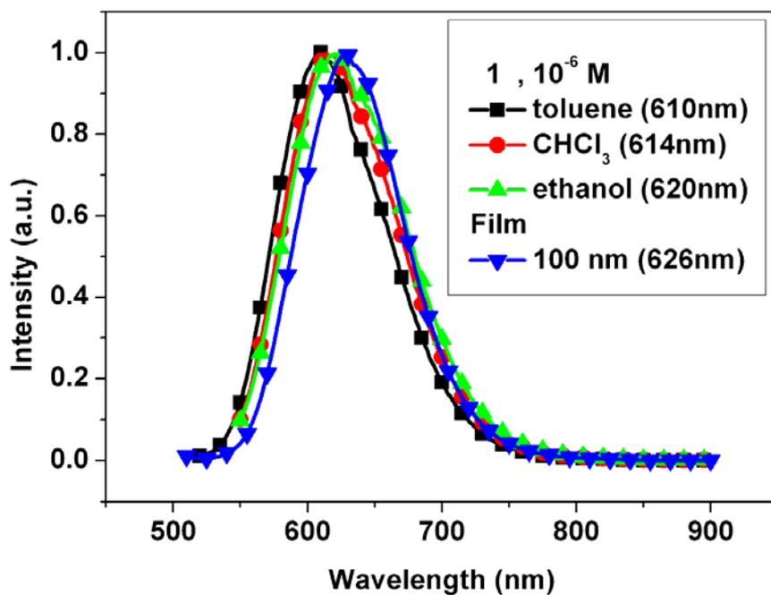
Figure S2. PL spectra of 1 in different solvents ( $1 \times 10^{-6}$  M).
