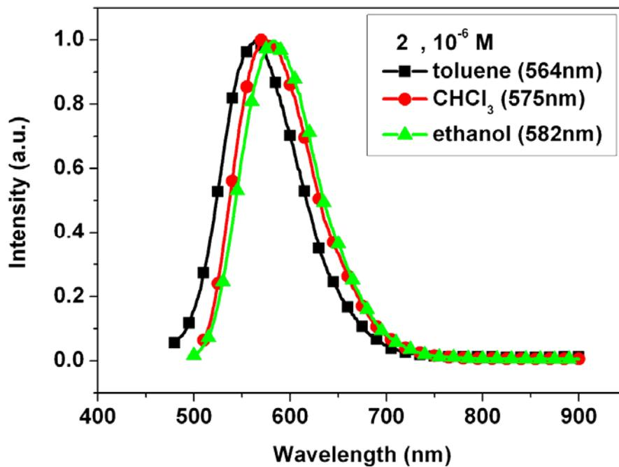
Figure S3. PL spectra of 2 in different solvents ( $1 \times 10^{-6}$  M).
