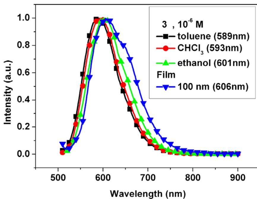
Figure S4. PL spectra of 3 in different solvents ( $1 \times 10^{-6}$  M).
