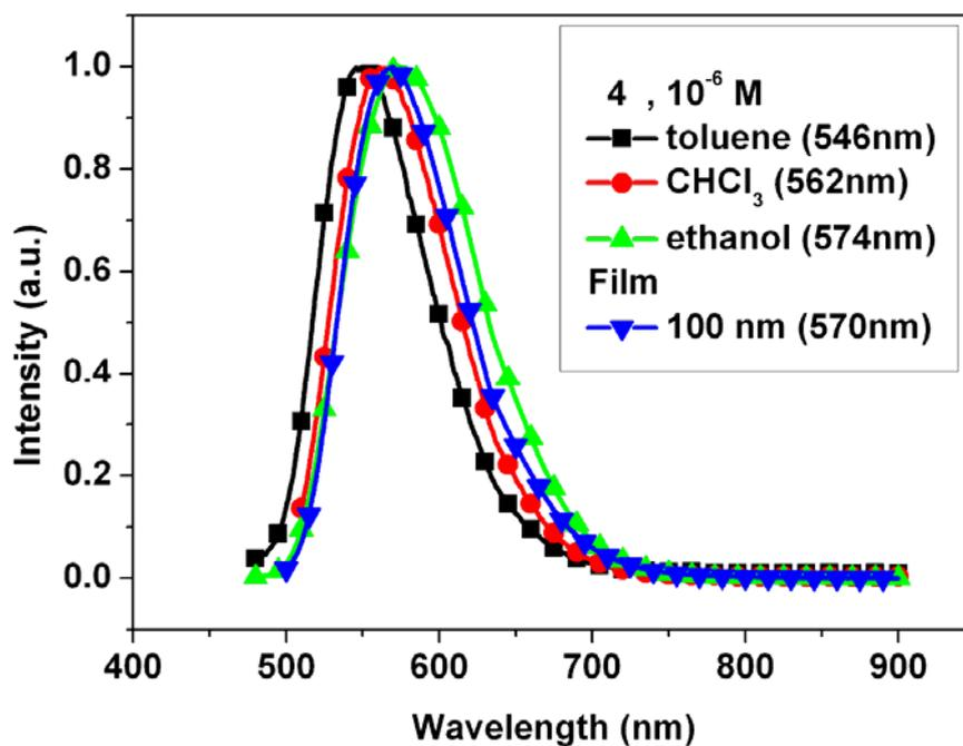
Figure S5. PL spectra of 4 in different solvents ( $1 \times 10^{-6}$  M).
