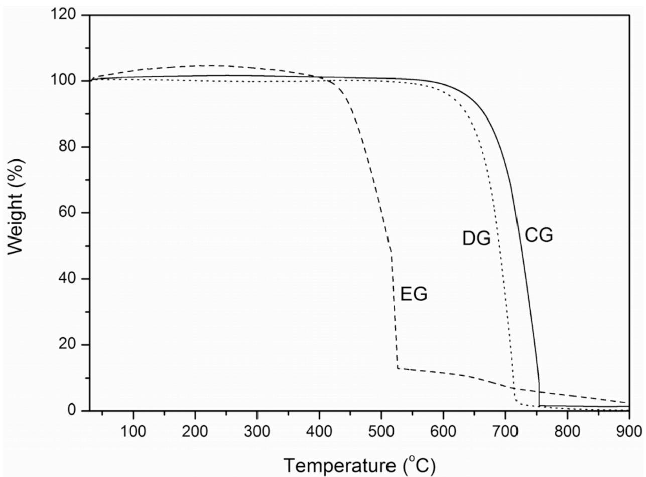
Thermogravimetric plot of oxidation of different graphene samples
