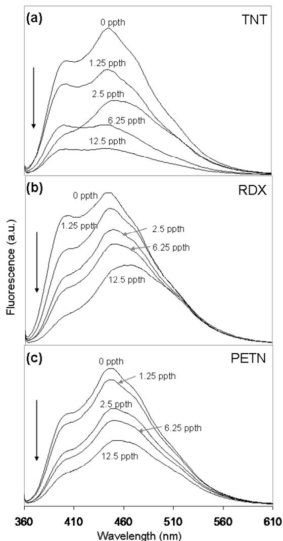
**Fig. S1** Solid-state fluorescence quenching behavior of **PSF2** on silica TLC plates in the presence of (a) TNT, (b) RDX, (c) PETN. The concentration of explosive is reported in pptb of explosive-to-polymer (pptb = parts per thousand by weight).
