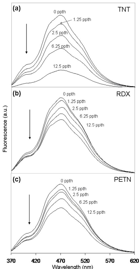
**Fig. S2** Solid-state fluorescence quenching behavior of **PSF3** on silica TLC plates in the presence of (a) TNT, (b) RDX, (c) PETN. The concentration of explosive is reported in pptb of explosive-to-polymer (pptb = parts per thousand by weight).
