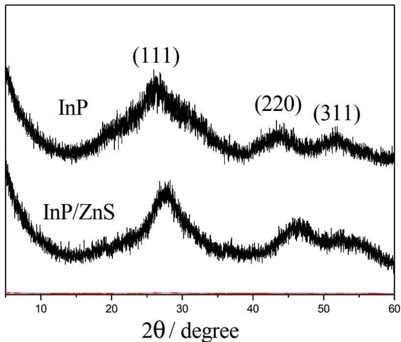
**Figure S.3:** The peaks in the XRD pattern of InP/ZnS core/shell samples shift to resemble the XRD pattern of ZnS and no mixed peaks of ZnS or InP NCs were found, indicating pure InP/ZnS particles. Narrow peak of InP/ZnS NCs comparing to InP NCs also showed the bigger size.
