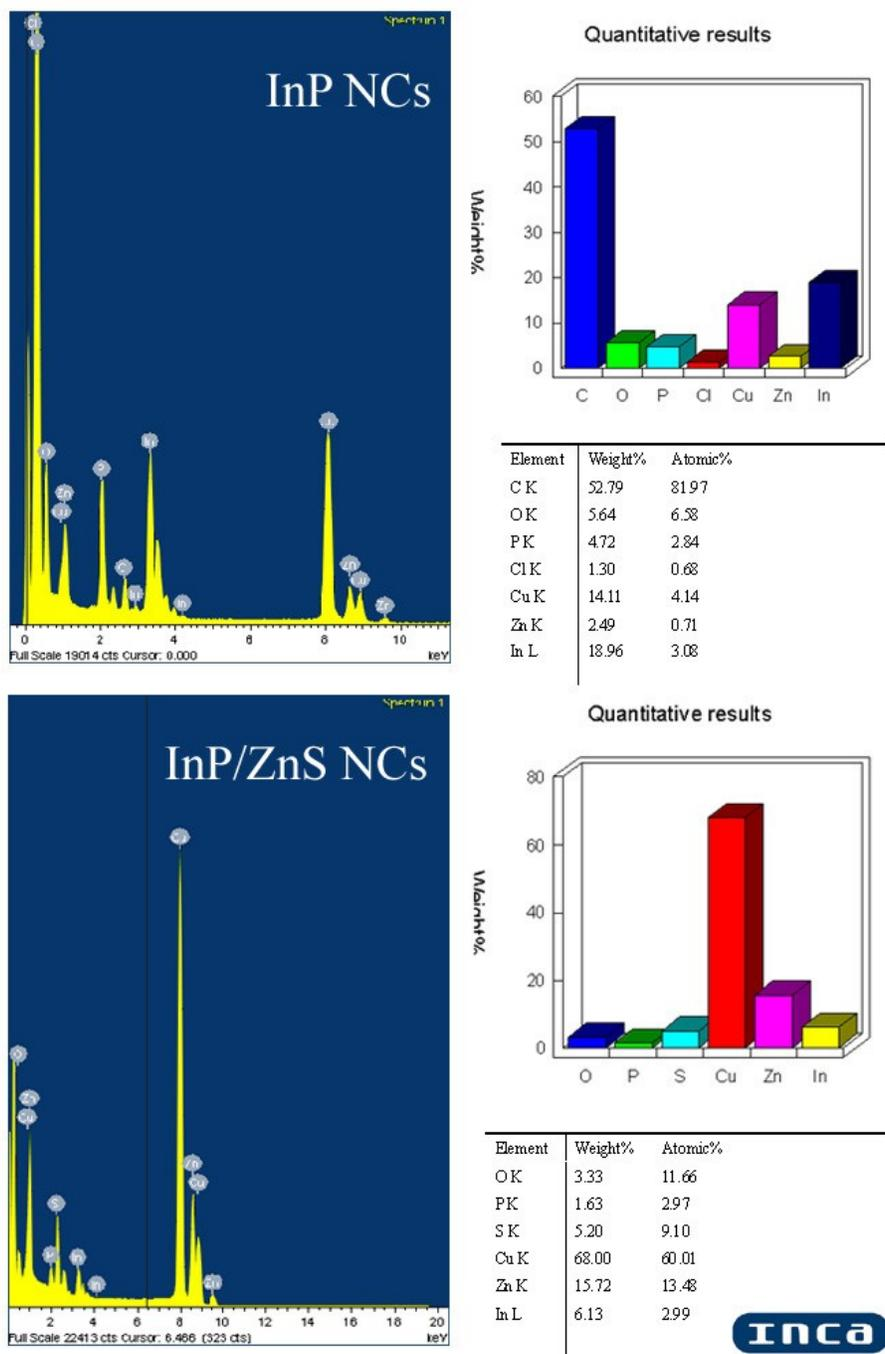
**Figure S.1:** The EDXS results for the zinc carboxylate capped InP NCs and InP/ZnS NCs. Elemental analysis showed a molar ratio In : P : Zn of  $\sim 1 : 0.93 : 0.23$  for a zinc carboxylate capped InP NCs and In : P : Zn : S of  $\sim 1 : 0.99 : 4.5 : 3.0$  for a InP/ZnS shelled NCs. The results indicated zinc rich particle surfaces.
