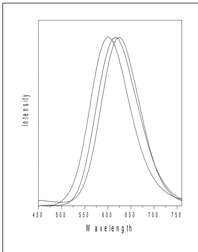
**Figure S.2:** The PL spectra of the InP NCs prepared with different concentrations of HDA. The reaction solution contained 0.1 mmol InCl<sub>3</sub>, 0.1mmol ZnUA and 0.1mmol SA. The amount of HDA for each sample is (from left to right): 0.5 mmol, 0.35 mmol, 0.2 mmol.
