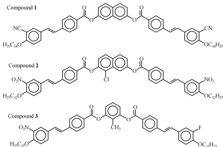
To 0.1 mol of central unit (2-methyl resorcinol or 2,7-dihydroxynaphthalene) dissolved in anhydrous tetrahydrofuran 2 ml of triethylamine, 20mg of DMAP and 0.022 mol of corresponding acid chloride was added. The reaction mixture was heated under reflux during 8 hrs. Then solvents were evaporated under diminished pressure. The crude product was chromatographed on silica gel and eluted by dichloromethane. Yields were varying from 55 to 70%.
