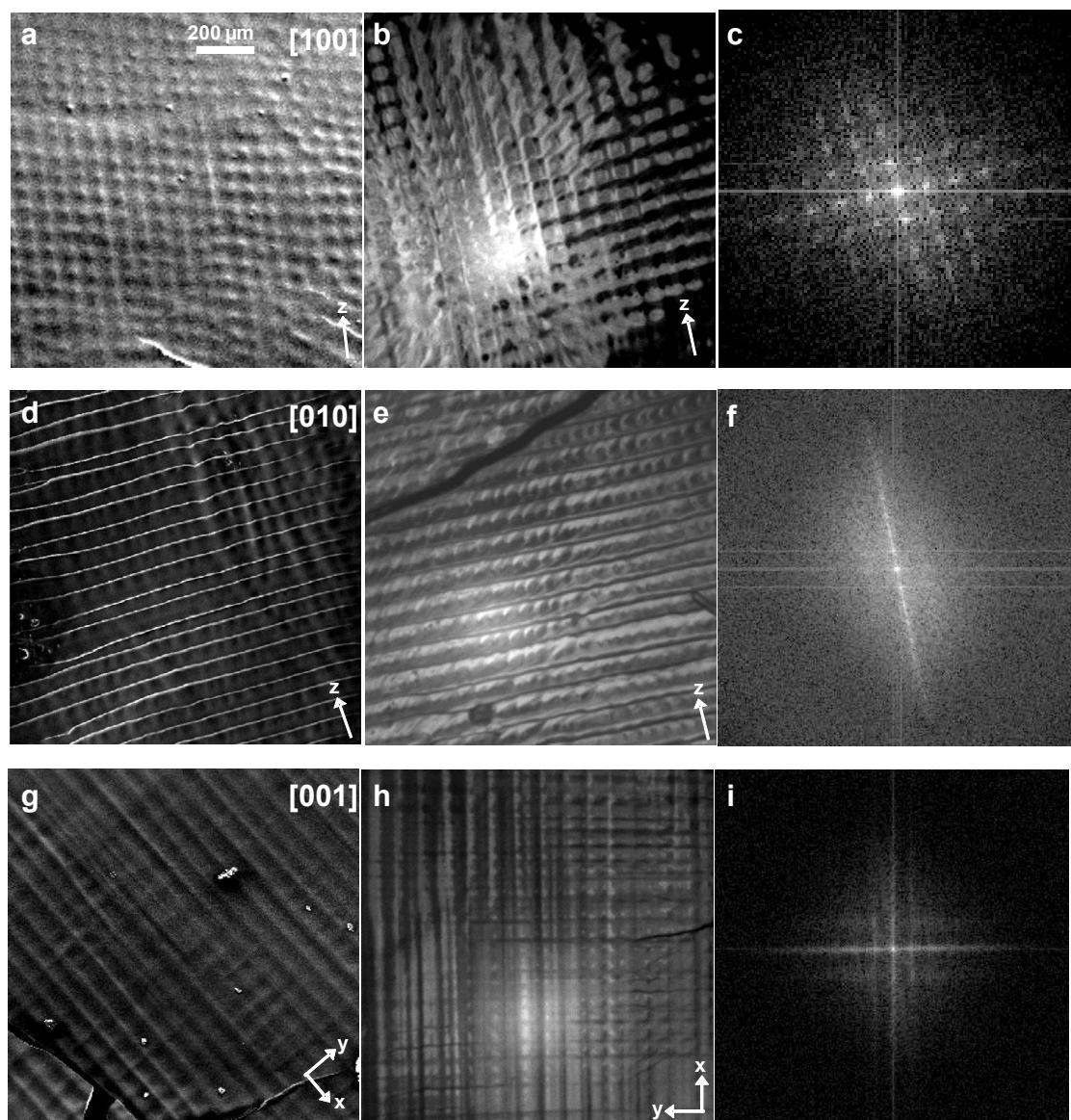
**Figure S3** Lattice structure induced by 2-beam configuration  $X_y+Y_z$ . Scanning electron and optical micrographs and Fourier transforms of the optical micrographs are shown for the [100] (a-c) [010] (d-f) and [001] (g-i) lattice faces. The scale bar in (a) applies to all micrographs.
