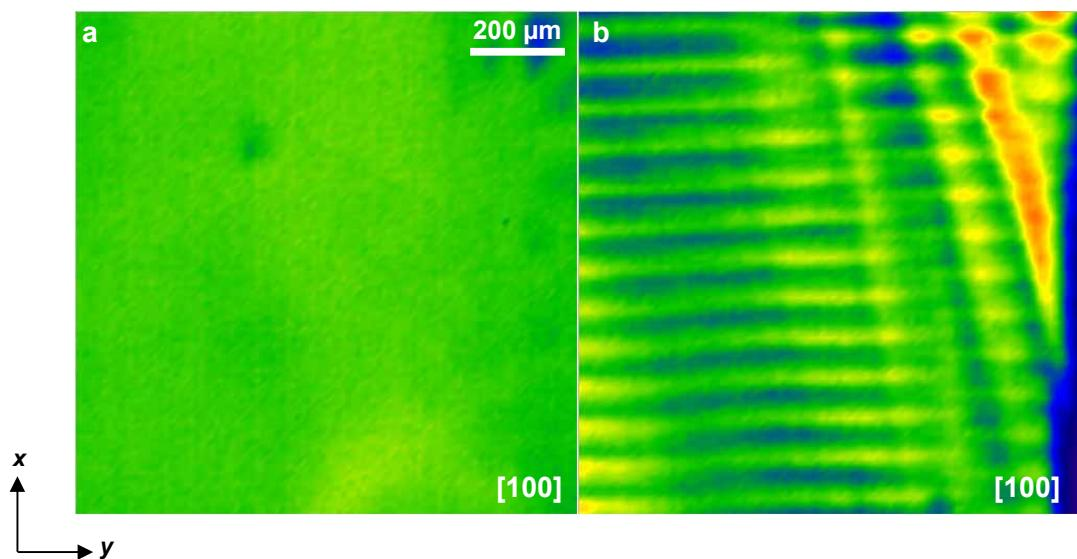
**Figure S2 Spatial intensity profiles of a passive beam X ( $> 550$  nm) in configuration X+Yz.** The initially uniform profile of beam X (a) develops a periodic modulation of bright stripes (b), confirming that it divides and propagates as self-trapped lamellae within the *same* periodic stack of lamellar waveguides induced by beam Yz. The same scale applies to both images.
