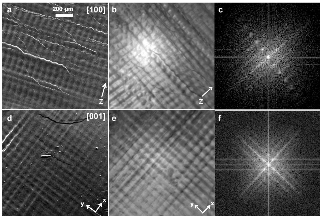
**Figure S4 Lattice structure induced by 2-beam configuration  $X_y+Y_x$**  Scanning electron and optical micrographs and Fourier transform of the optical micrograph are shown for the (a-c) [100] and (d-f) [001] lattice faces. The scale bar in (a) applies to all micrographs.
