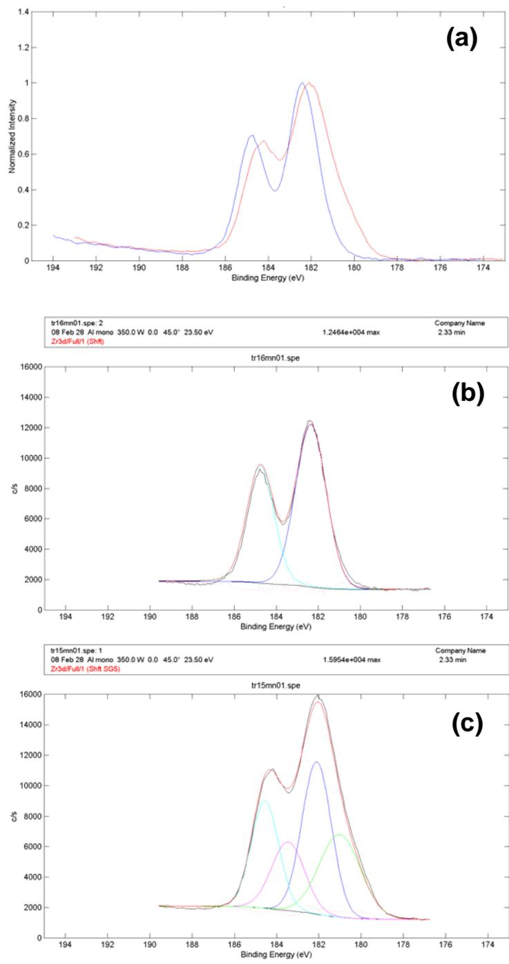
**Figure 5** (a) Zr3d XPS spectra of a YSZ dense pellet (sample no reduced - blue line-) and (sample reduced -red line-). The observed shoulder together with the use of four peaks (c) instead of two (b) to properly fit the spectra indicate the presence of Zr(III).
