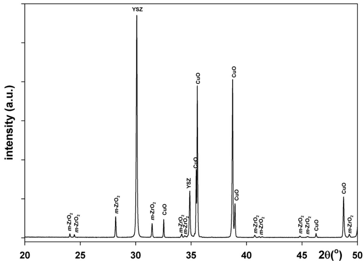
**Figure 1** XRD pattern for a composite YSZ-CuO (1:1 weight), after firing in air, at 1000°C for 3h. YSZ powder was previously annealed at 1200°C for 15h.
