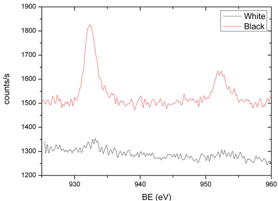
**Figure 4** XPS spectra of Cu<sub>2p</sub> core level electron of bulk YSZ (**grey line**: white zone in YSZ sample; **red line**: dark zone in Cu-YSZ interface).
