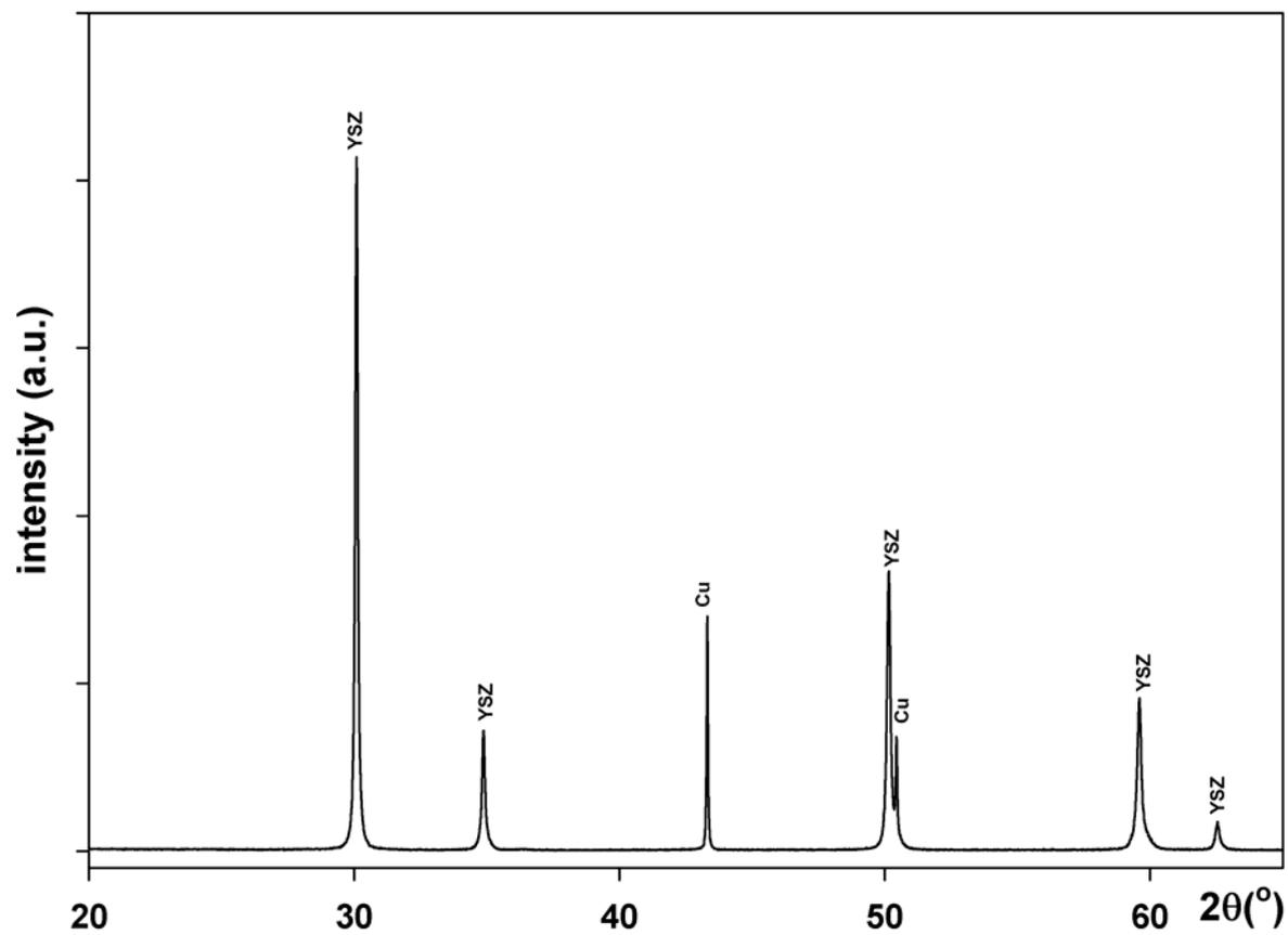
**Figure 2** XRD pattern for a cermet YSZ-Cu (YSZ:CuO=3:1 weight), after firing at 950°C, under humidified 5% $H_2$ -Ar, for 3h. No peaks from  $m$ - $ZrO_2$  were observed.
