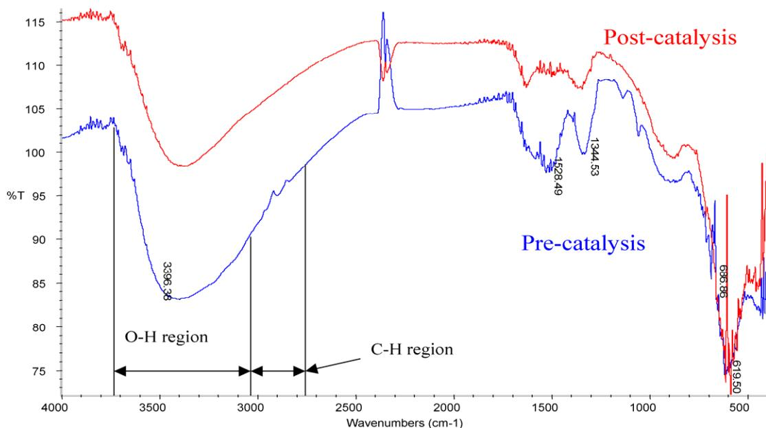
**Figure S4** FTIR for sample C4, ox-en (1:1) capped CoFeO<sub>4</sub> nanoparticles
