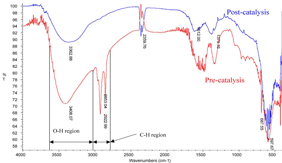
**Figure S5** FTIR for sample C2, CTAB capped CoFe<sub>2</sub>O<sub>4</sub> nanoparticles
