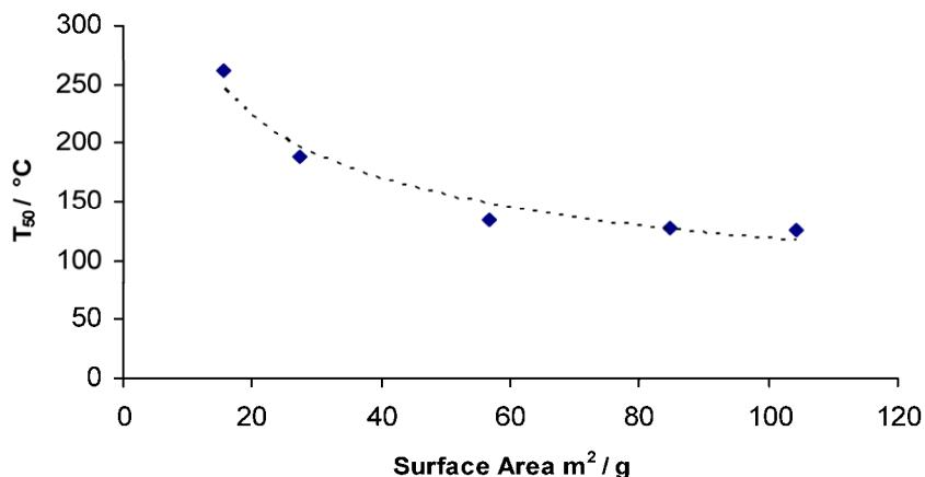
**Figure S9**  $T_{50}$  versus BET surface area for samples C4, C5, C6 and C7. The line is a guide to the eye.
