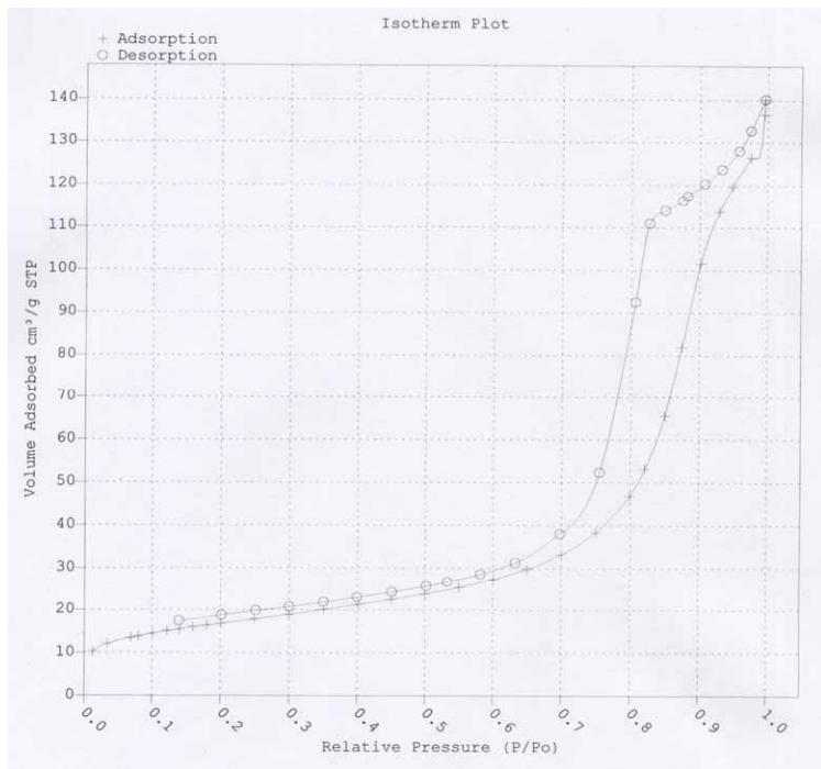
**Figure S3** N<sub>2</sub> absorption and desorption isotherms for sample C10, 15 nm particles
