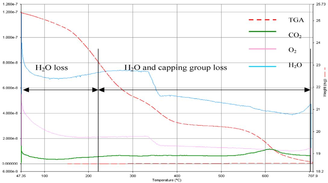
**Figure S7** TGA-MS for sample C2, CTAB capped CoFe<sub>2</sub>O<sub>4</sub> nanoparticles
