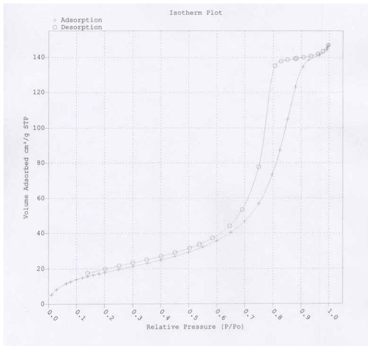
**Figure S2** N<sub>2</sub> absorption and desorption isotherms for sample C2, 12 nm particles
