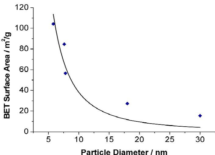
**Figure S8** BET surface area versus particle size for samples C4, C5, C6 and C7. The data is fitted to the function  $y = A x^{-2}$  where A is  $3820 \pm 377$ .
