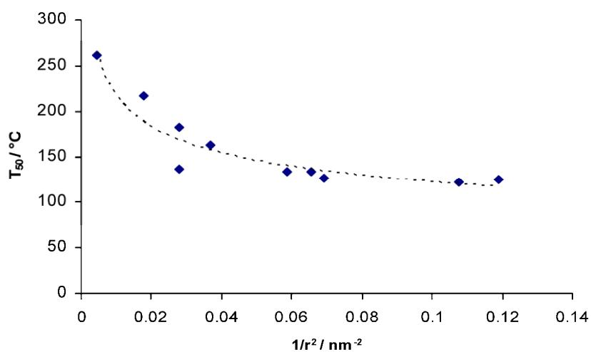
**Figure S10**  $T_{50}$  versus  $1/r^2$  for samples C1-10. The line is a guide to the eye.
