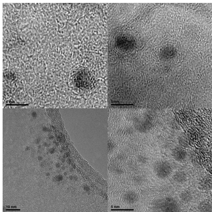
**Figure S1** TEM images for sample C6, 5.8 nm ox-TEA capped nanoparticles.
