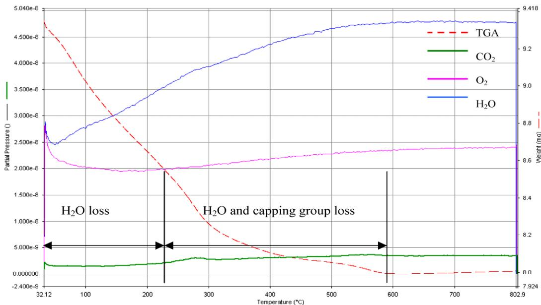
**Figure S6** TGA-MS for sample C3, ox-en (2:1) capped nanoparticles. The above is representative of the TGA-MS for samples C4, C5 and C6
