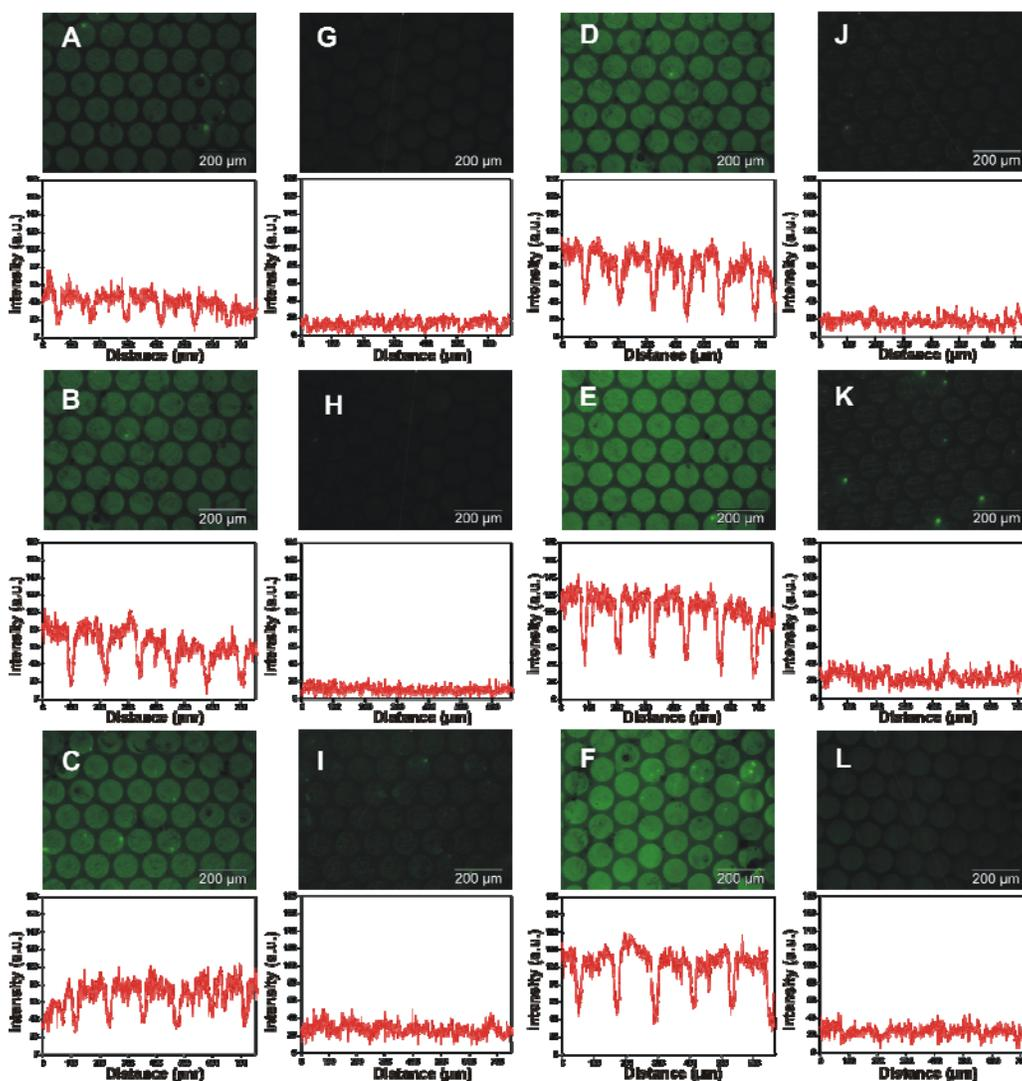
**Fig. 2** Fluorescence microscopy images (884 μm x 666 μm) of 100 μm Atto520 printed dots onto **IM** (A,B,C,D,E,F) and **NH<sub>2</sub> SAMs** (G,H,I,J,K,L) for 5 min, 15 min, 30 min, 50 min, 1h and 2h.
