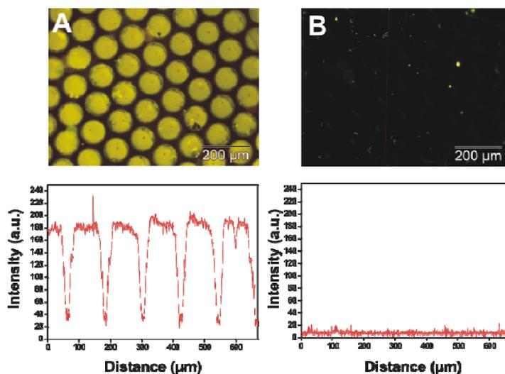
**Fig. 4** Fluorescence microscopy image (884 μm x 666 μm) of boc-ADF (1 mM in acetonitrile) printed 100 μm diameter dots onto **IM SAM** for 20 min before (A) and after (B) THF rinsing.
