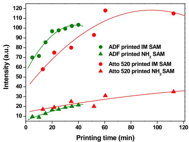
**Fig. 1** Reaction rate of ADF and Atto520 printed onto **IM SAM** and **NH<sub>2</sub> SAM**
