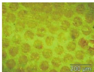
**Fig. 3** Fluorescence microscopy image (884  $\mu\text{m}$  x 666  $\mu\text{m}$ ) of Octadecylamine (1 M in acetonitrile) printed 100  $\mu\text{m}$  diameter dots onto **IM SAM** for 1h. The remaining area was filled by exposing samples to Atto520 in solution overnight (0.1mM in MilliQ water).
