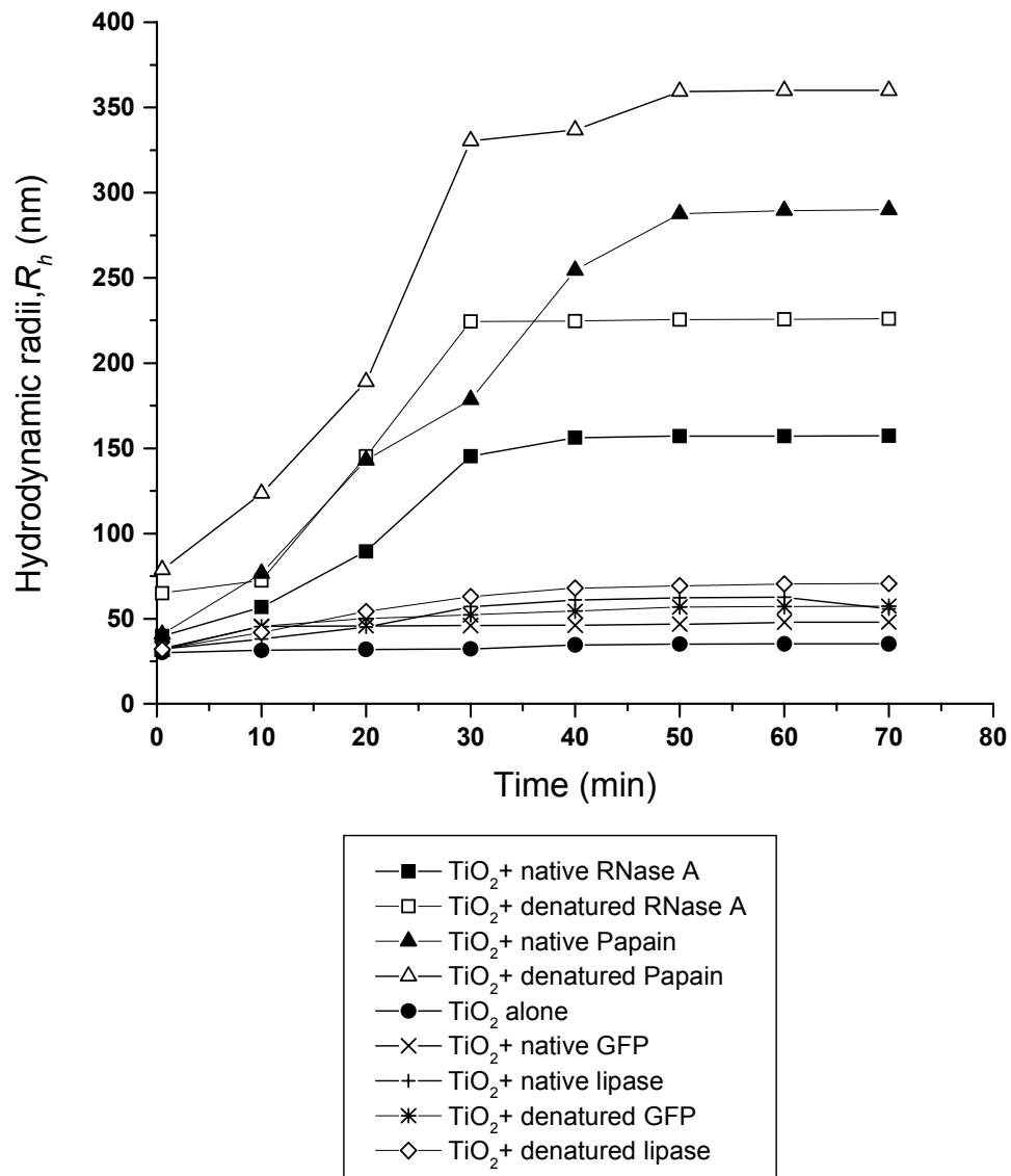
**Fig. S1** The size distribution of  $\text{TiO}_2$  particles and protein sample (both native and thermally denatured) during association by DLS after different time interval.
