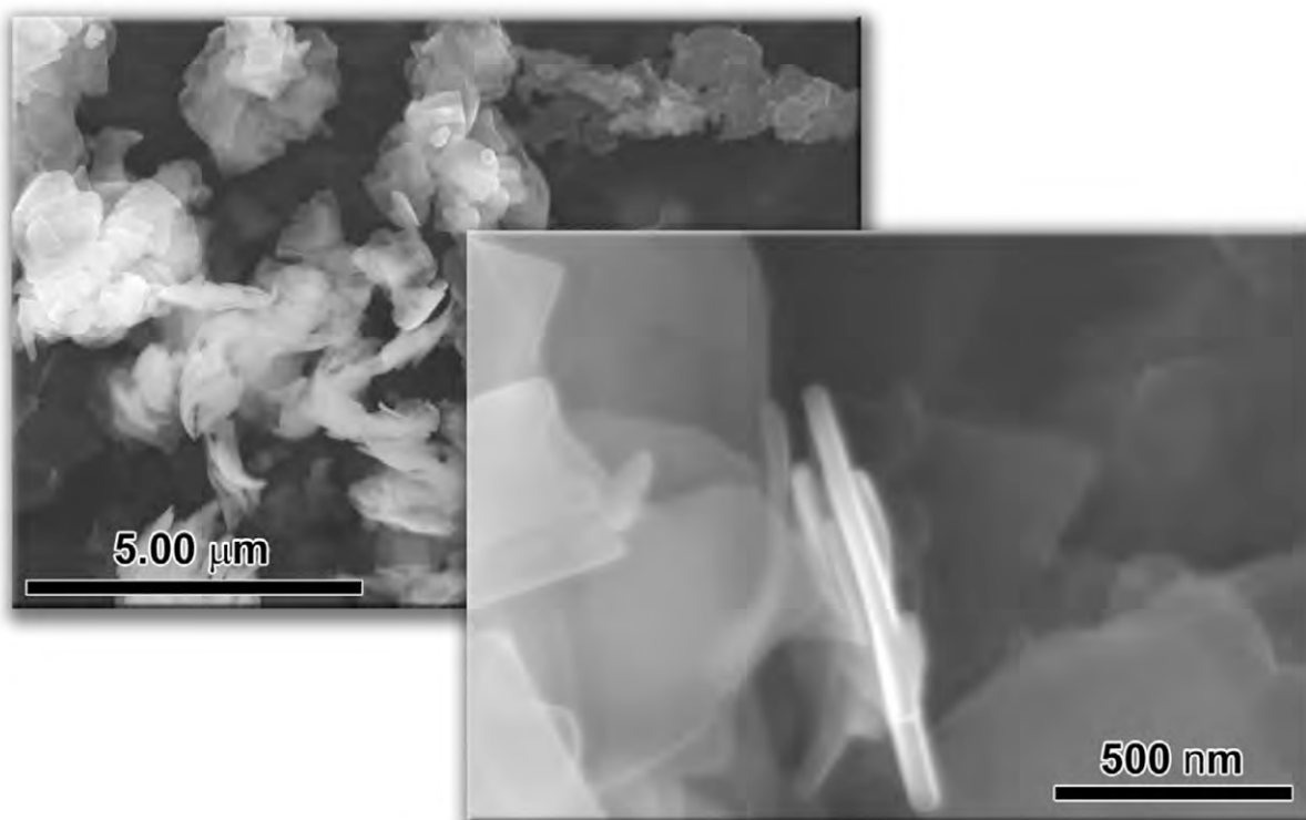
Figure S17 - SEM pictures of [\text{Sm}(\text{H}_2\text{cmp})(\text{H}_2\text{O})] (5).
