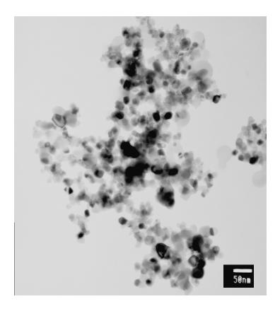
**Figure 1S** TEM image of RB5 supernatant solution, after 12 hours of UV-TiO $_2$ -paper irradiation (365nm, 23W m $^{-2}$ ).
