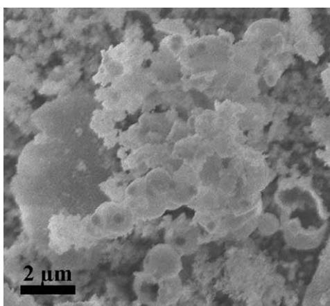
**Figure S5.** SEM images of the siliceous hollow microspheres.
