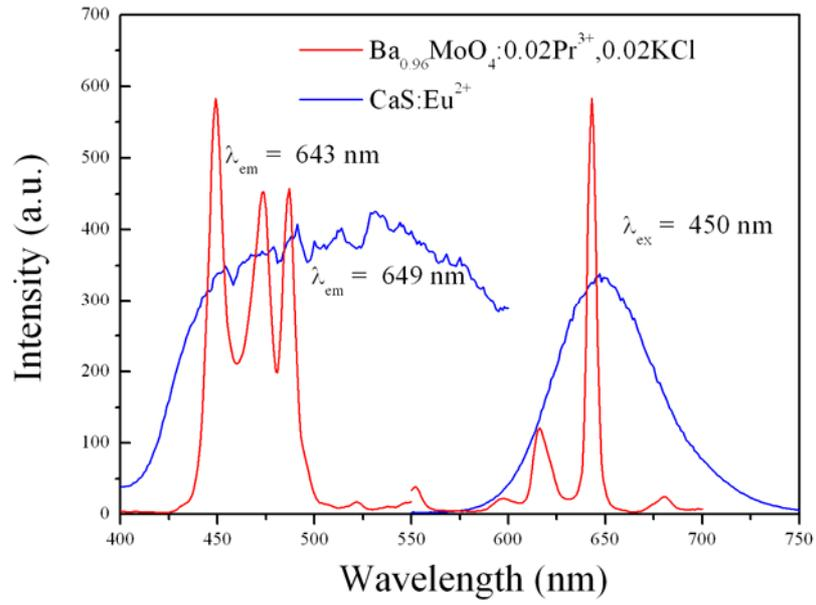
Fig. S4. The excitation spectra of  $\text{Ba}_{0.98}\text{MoO}_4:0.02\text{Pr}^{3+}, 0.02\text{KCl}$  ( $\lambda_{\text{em}} = 643 \text{ nm}$ ) and  $\text{CaS:Eu}^{2+}$  ( $\lambda_{\text{em}} = 649 \text{ nm}$ ), the emission spectra of  $\text{Ba}_{0.98}\text{MoO}_4:0.02\text{Pr}^{3+}, 0.02\text{KCl}$  and  $\text{CaS:Eu}^{2+}$  ( $\lambda_{\text{ex}} = 450 \text{ nm}$ ).
