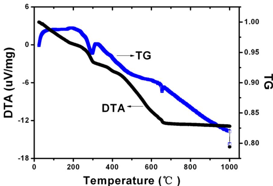
Fig. S1 TG/DTA curves of the BMO precursor in synthetic air, using a constant heating rate of  $10^\circ\text{C}/\text{min}$
