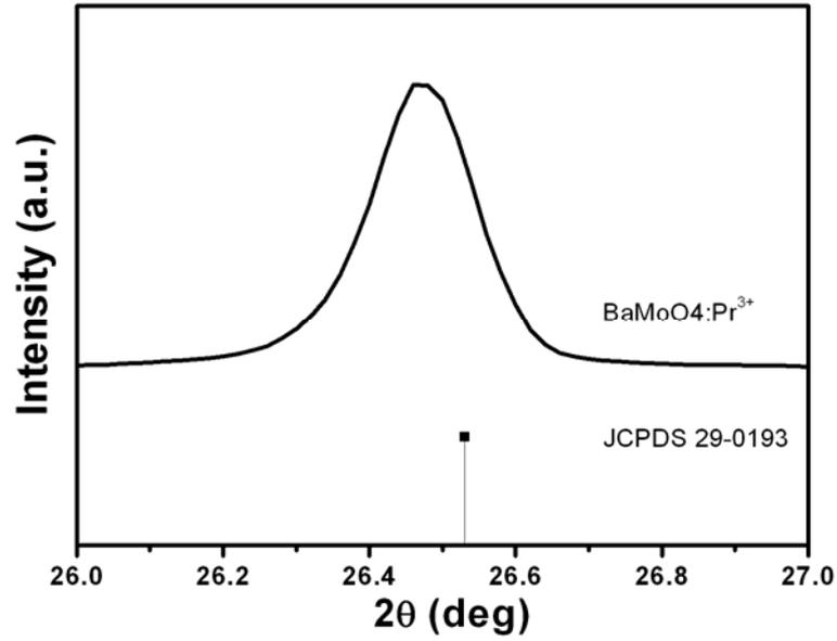
Fig. S2. Enlarged version of XRD patterns of BaMoO<sub>4</sub>: Pr<sup>3+</sup> phosphor sintered at 800°C from 26°C to 27°C.
