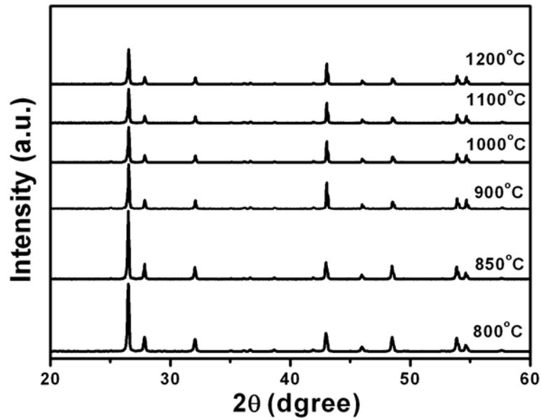
Fig. S3. XRD patterns of as-prepared products sintered in different temperatures.
