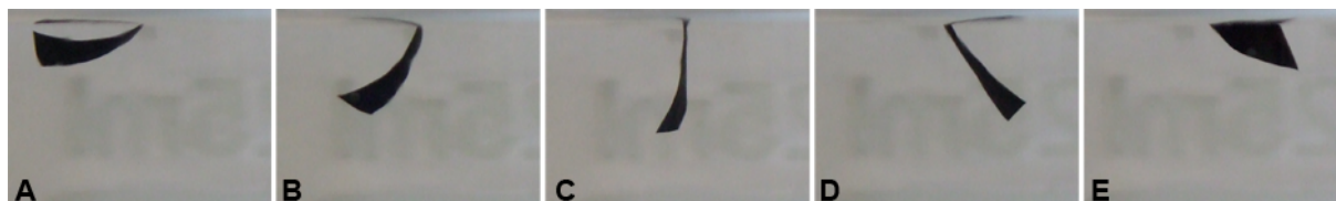
Fig. S4 Optical images recorded during the process of actuator 2 bending in 1.0 \text{ mol L}^{-1} \text{ LiClO}_4 aqueous solution by voltammetric scanning in the potential range of -1.0 \text{ V} (A) and +1.0 \text{ V} (E), versus SCE at a scan rate of 50 \text{ mV s}^{-1} ; the actuators were held with the inverse opal side to the right.
