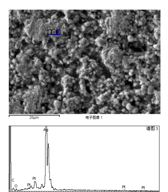
The above two figures are the SEM micrograph and EDX spectrum of the polished surface of the  $Ag/BST/PbO-B_2O_3$  composite with Ag volume fraction f=0.18. The EDX spectrum implies that the region being detected has composition similar to pure Ag and this further confirms the distribution and aggregation of Ag.
