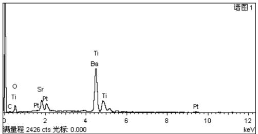
The above two figures are the SEM micrograph and EDX spectrum of the polished surface of the Ag/BST/PbO- $B_2O_3$  composite with Ag volume fraction f=0.18. The EDX spectrum implies that the region being detected has composition similar to pure BST.
