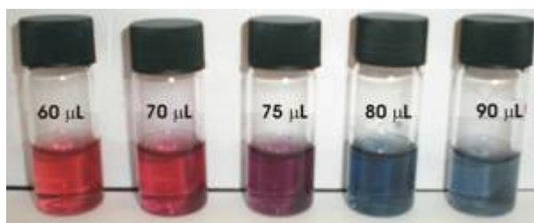
Figure S3: Digital image of 5 samples of gold nanoparticle suspensions to which different amounts of HNO 3 were added to induce rapid aggregation. An instantaneous dramatic colour change characteristic of aggregation in the suspension is noted as the volume of acid added is increased. In the last two samples, large aggregates were observable with the naked eye.
