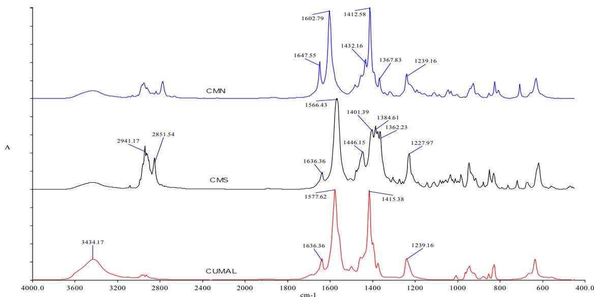
**Figure S2.** FT-IR spectra of copper(II) (meth)acrylate complexes, **CUMAL**, **CMS** and **CMN**
