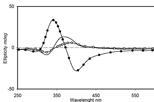
Figure S6. CD spectra of P8R as prepared film (—), and annealed at isotropic temperature and after cooled down at 10°C/min (—○—) and 1.2°C/min (—●—).
