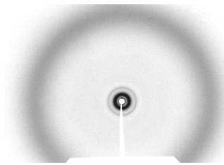
Figure S3. X-Ray pattern of a sample of P8S cooled at 1°C/min.
