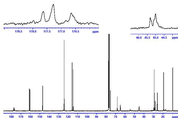
Figure S1.  $^{13}\text{C}$  NMR of the polymer P4S. Inset of the region corresponding to  $\text{C}=\text{O}$  and  $\text{CH}_2$  (methylenic chain group) is included.
