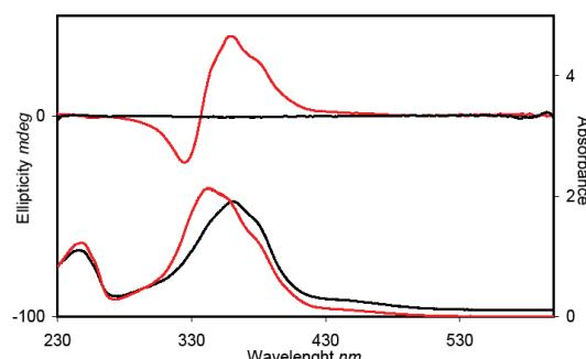
Figure S5. UV-vis (down) and CD spectra (up) of P8R in DCM solution (—) and in DCM/hexane solution (—).
