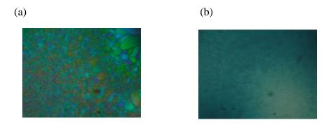
ESI Fig. S1 Photomicrographs of (a) the blue phase at 71°C of compound 1 and (b) that after being sheared.
