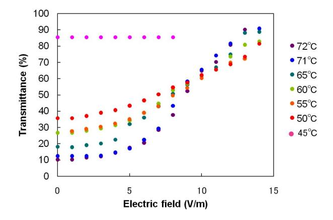
ESI Fig. S3 Temperature dependence of optical transmittance of compound **1** in the BP as a function of an AC field at a frequency of 0.1 Hz.
