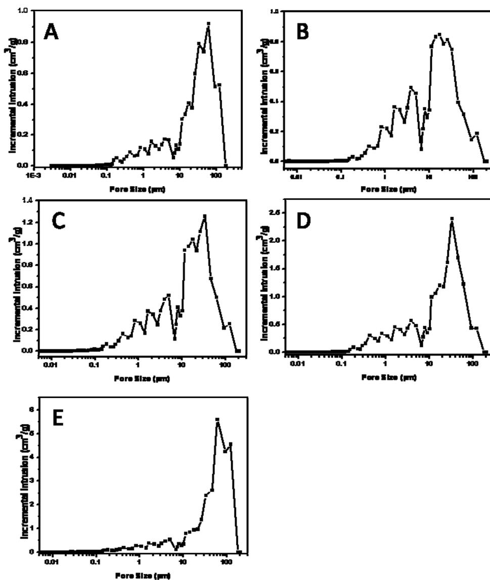
**Fig. S2** Pore size distribution of emulsion-templated porous SCMC as measured by mercury intrusion porosimetry at different volume percentage of internal phase in the emulsions. (A) 0 v/v %. (B) 20 v/v %. (C) 40 v/v %. (D) 60 v/v %. (E) 75 v/v %.
