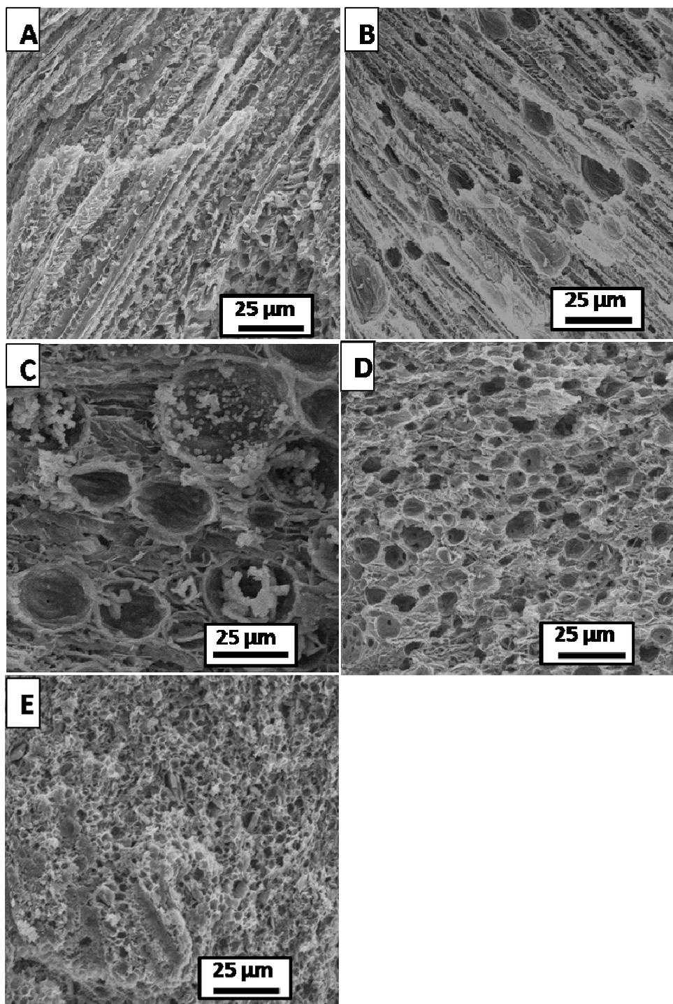
**Fig. S4 Porous zirconia/PVA composites with tuned pore morphology and porosity, prepared from emulsion-templated PVA beads. (A) 0 v/v %. (B) 20 v/v. (C) 40 v/v %. (D) 60 v/v. (E) 75 %.**
