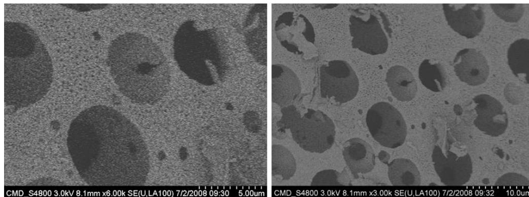
**Fig. S3** The porous surface of silica beads calcined from PVA-HS30 beads.
