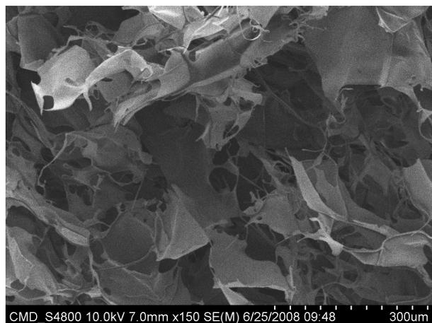
**Fig. S1** The random porous structure of SCMC by freezing a 1wt % SCMC aqueous solution in a freezer and then freeze drying.
