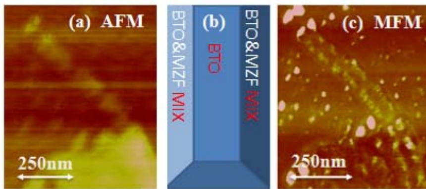
**Figure S2.** AFM (a) and MFM(c) measure from a rod; and (b) is the schema of the phase distribution in one rod.
