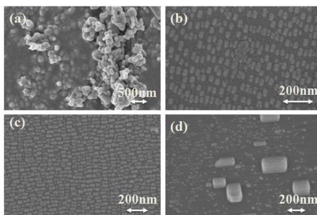
**Figure S3.** SEM images of the sample taken at different reaction time to understand the growth process: (a) is the mixed raw reagent powders; (b) is after reacting for 10min; (c) is after reacting for 20min; and (d) is after reaction for 60min.
