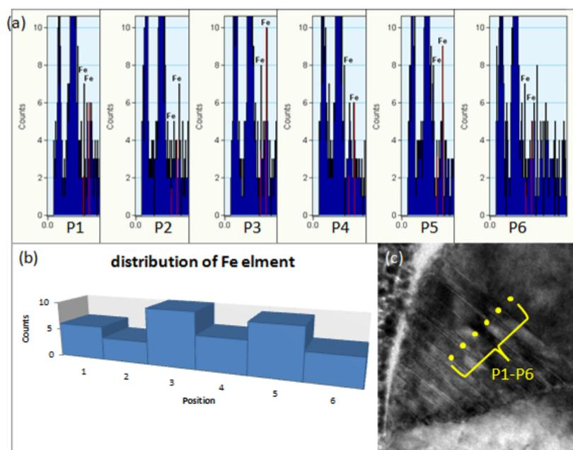
**Figure S1.** (a) EDS spectra were taken from six different points shown in (c) HRTEM image. (b) Iron element distribution profile base on these spectra shown in (a).
