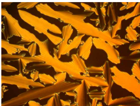
Figure S2. Polarised light optical photomicrograph of the SmA phase of 8b at 179 °C (magnification x 200).
