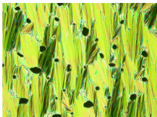
Figure S1. Polar (bistable, ferroelectric) switching of the SmC* phase of compound 6c at 110 °C as seen between crossed polarizers (6 \mu\text{m} ITO cell, EHC, Japan).
