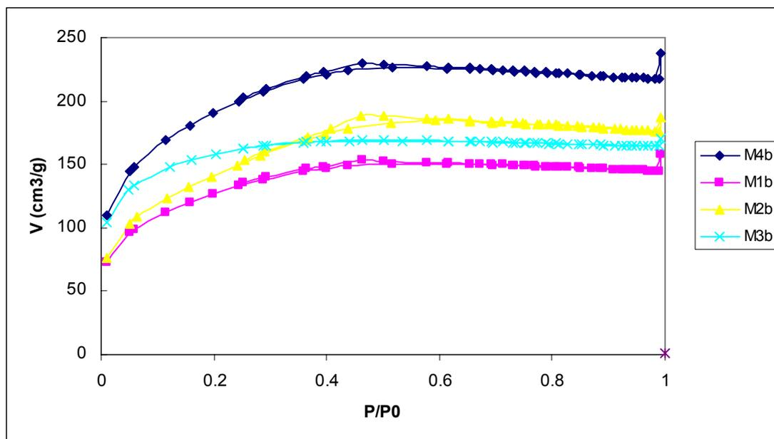
Figure S<sub>14</sub>. Nitrogen adsorption desorption of hybrid materials prepared under basic conditions
