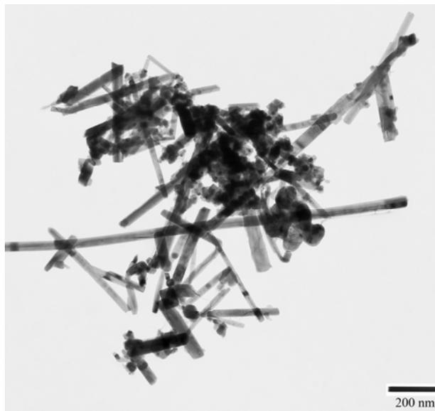
Supplemental Figure 3: TEM micrograph of the product of annealing hexagonal potassium tungstate nanorods in 10% H<sub>2</sub> for 1 h.
