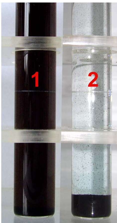
Fig. S5 The \text{CaCO}_3 surface-modifying CR and MB material was prepared by adding CR and MB into a \text{CaCO}_3 powder liquid, thus both CR and MB were adsorbed on the outside surface of \text{CaCO}_3 powder particles. The suspending substance was washed with distilled water (1). The CR-MB conjugate – \text{CaCO}_3 hybrid was prepared according to the present work and washed with distilled water (2). The concentrations were 200\ \mu\text{M} CR, 400\ \mu\text{M} MB and 0.06\% \text{CaCO}_3 and both the water-washing liquids were settled naturally for 30 min.
