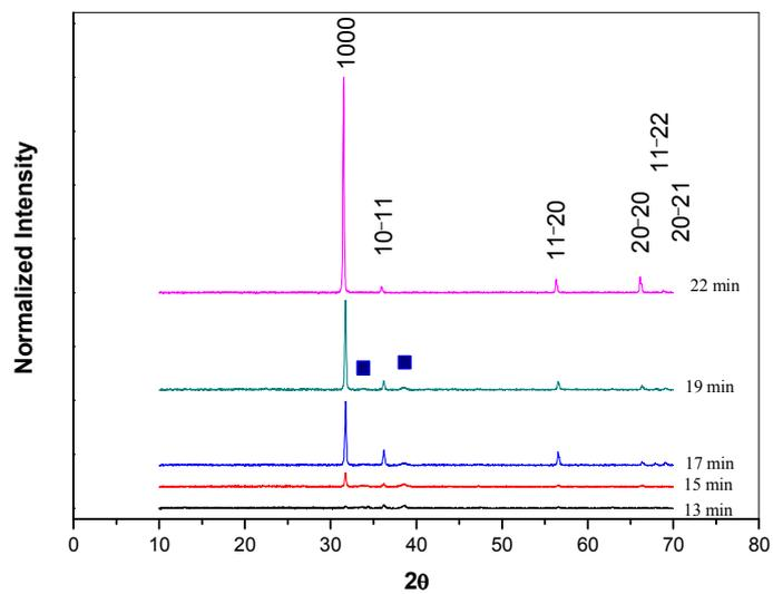
ESI 2; Fig. 1: XRD of samples prepared by varying time of irradiation (● -  $\text{Zn}_5(\text{CO}_3)_2(\text{OH})_6$ ; ■ - from the instrument)
