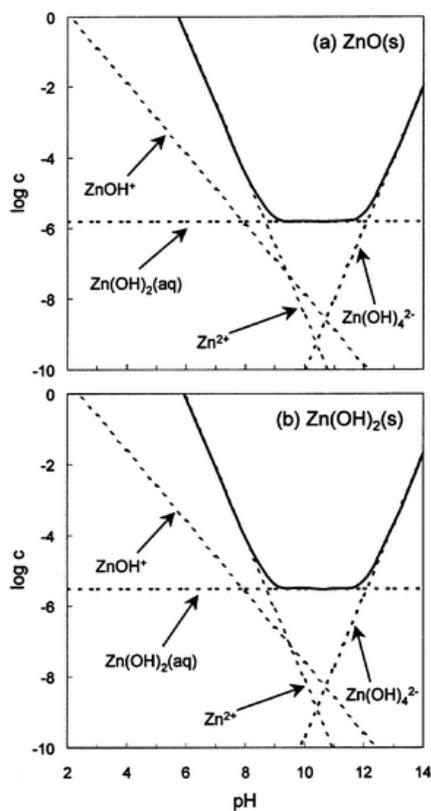
ESI 6; Fig. 1: Phase stability diagrams for the ZnO(s)-H<sub>2</sub>O (a) and Zn(OH)<sub>2</sub>(s)-H<sub>2</sub>O (b) systems at 25 °C as a function of pH. An equilibrium between Zn(OH)<sup>3-</sup> and the solid phase is out of the range (Taken from references mentioned in 36. Thermodynamic data of the phases can also be found therein).
