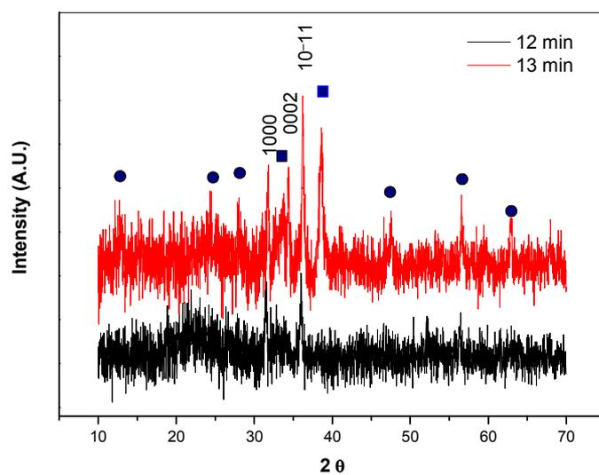
ESI 2; Fig. 2: XRD of sample prepared by 12 and 13 min of MW irradiation (● -  $\text{Zn}_5(\text{CO}_3)_2(\text{OH})_6$ ; ■ - from the instrument)
