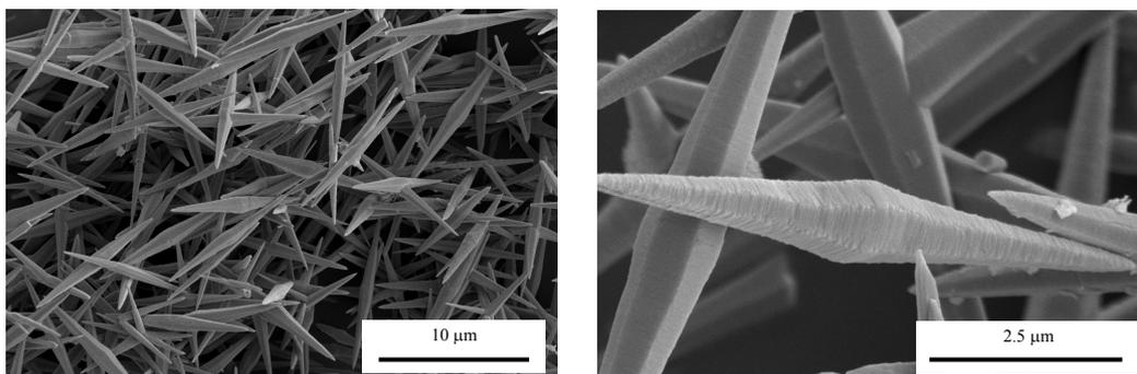
**ESI 1; Fig. 1:** SEM of sample prepared by 20 min. of MW irradiation between 40 mL each of 10 mM zinc nitrate and 10 mM urea (1:1)
