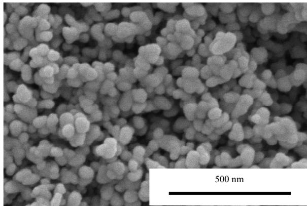
**ESI 5; Fig. 1:** SEM image of 500 °C calcined product of the ammonium carbamate and zinc nitrate reaction.
