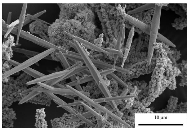
**ESI 1; Fig. 2:** SEM of sample prepared by 20 min. of MW irradiation between 40 mL each of 100 mM zinc nitrate and 100 mM urea (10:10)
