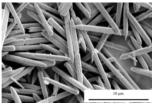
**ESI 4; Fig. 1:** SEM of sample prepared by irradiating the already microwaved solution (150W 14 min) for 18 min. after adjusting the pH to 10 (\*). The surface texture is rough due to the dissolution of the particles. (size ~13 μm)
