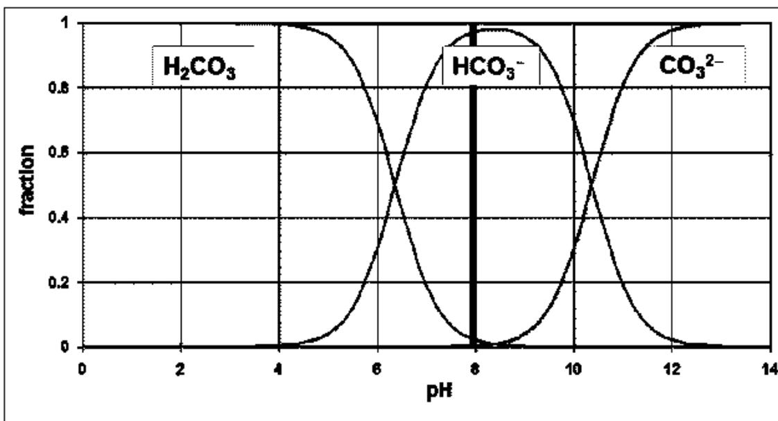
ESI 7; Fig. 1: Carbonate-bicarbonate phase distribution diagram. Solubility product of carbonate at pH 8 is  $8.5 \times 10^{-4}$ .
