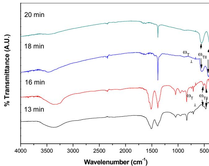
ESI 3; Fig. 1: FTIR spectra of ZnO micro-javelins prepared at various reaction times
