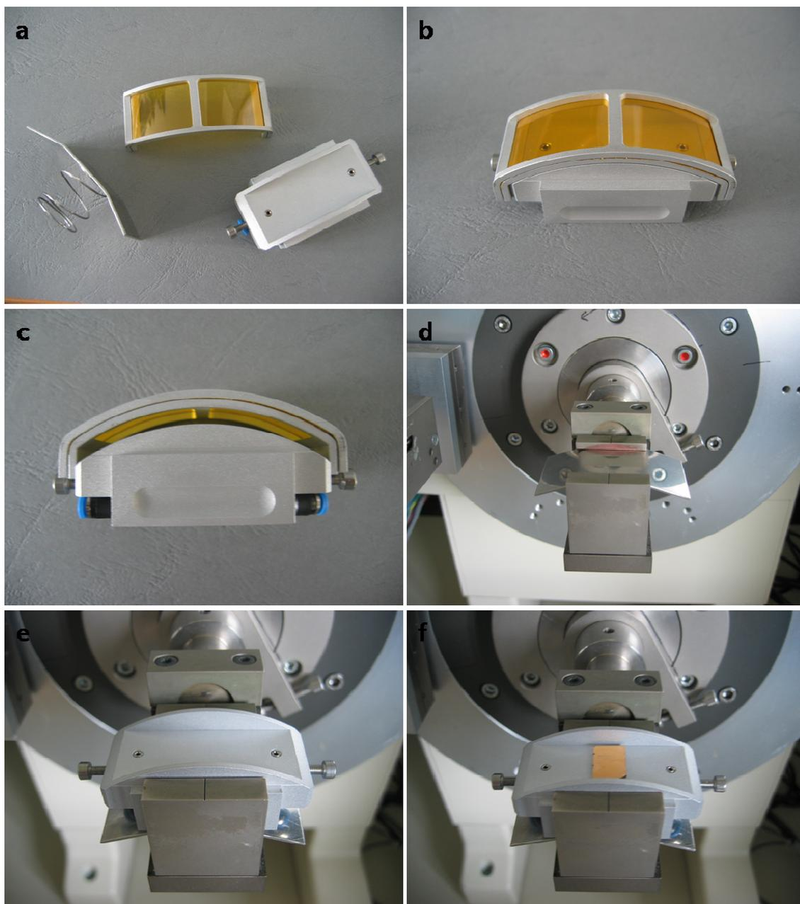
**Figure S1.** Pictures of sample cell for Sorption@XRD measurements (a-c) and the positioning of the cell into the Scintag XDS 2000 X-ray diffractometer (d-f).
