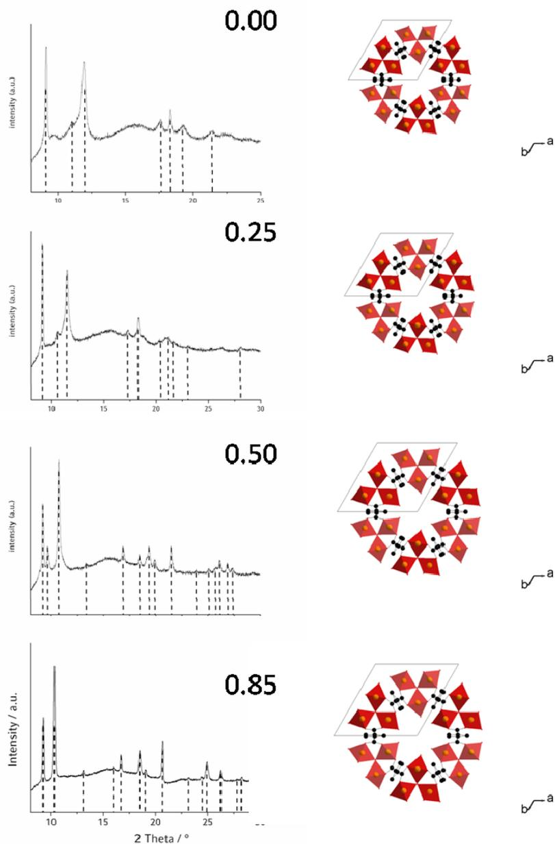
**Figure S3.** Comparison of the measured X-ray patterns under the given relative pressures with the simulated patterns. Parameters of indexation are given in Table 1. The size of the unit cell as a function of relative pressure is depicted schematically.
