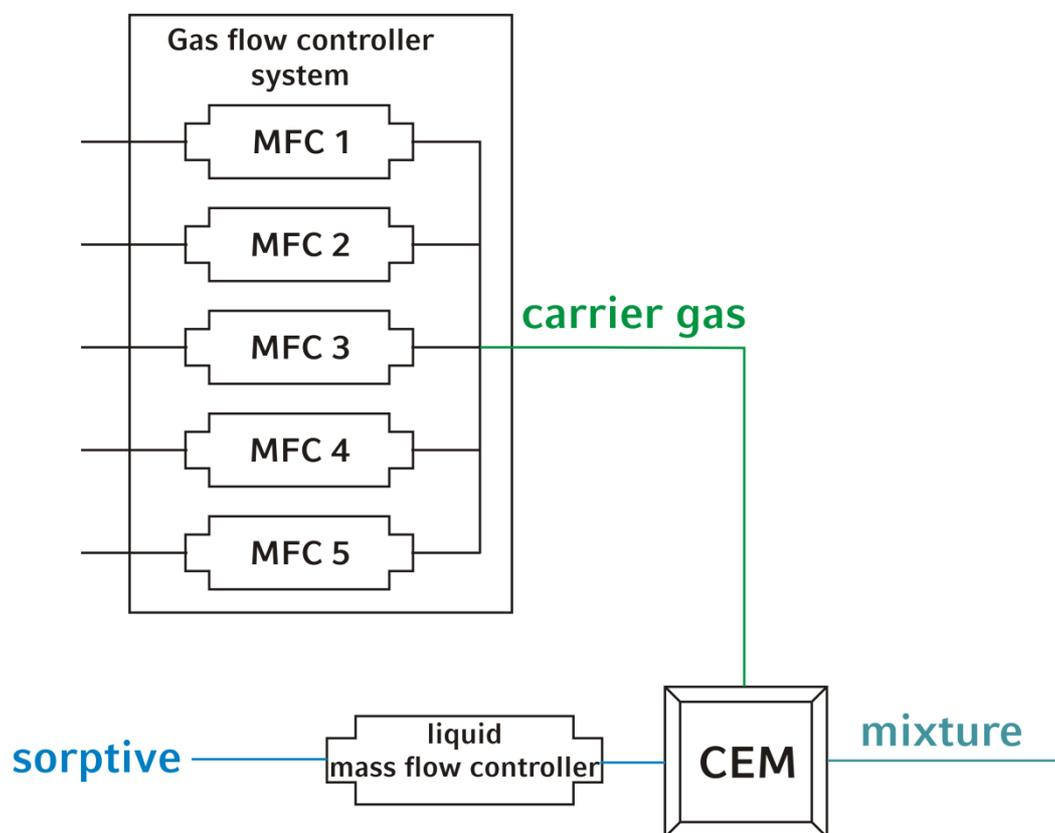
**Figure S2.** Experimental setup of the flow controlling system employed in this work, consisting of the gas flow controlling system, a liquid mass flow controller and a controlled evaporation mixer (CEM).
