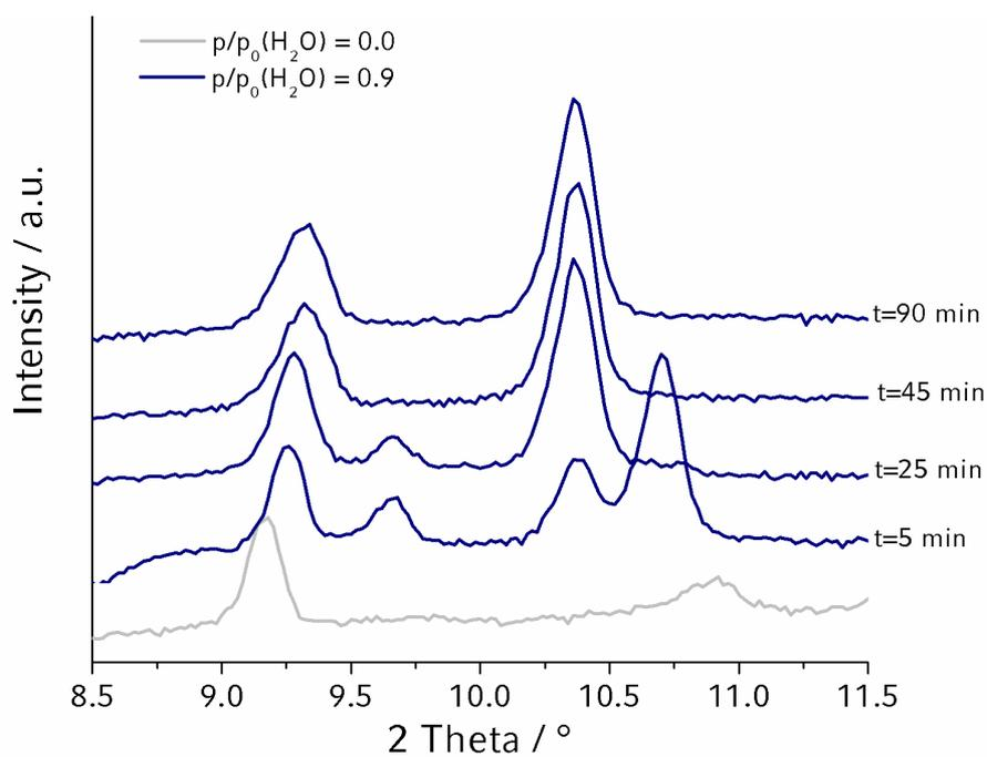
**Figure S4.** Evolution of structural changes of dry MIL-88B exposed to a relative pressure of water of 0.9.
