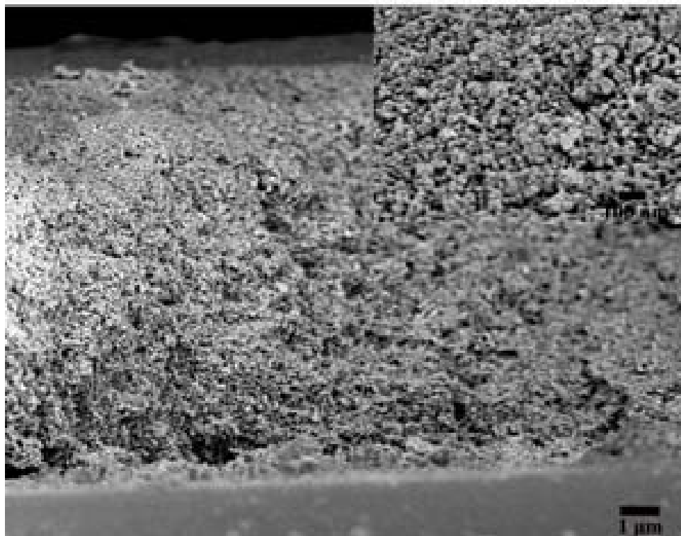
Figure S8. Cross sectional view of a ZnO nanoparticles photoanode. Inset: High magnification SEM image of the ZnO nanoparticles.
