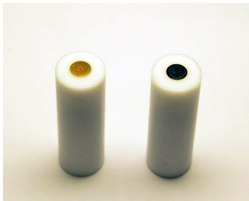
Fig. S1 The images of graphene oxide on gold disk electrodes before (left) and after (right) the electrochemical reduction.
