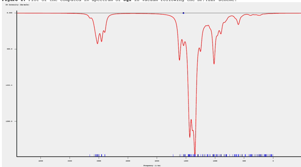
Figure 1. Plot of the computed IR spectrum of SQ1 in vacuum following the BP/TZ2P scheme.
