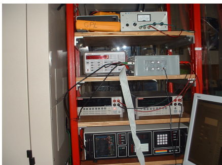
Fig. S4 Experimental set up for electrical measurements using the Van der Pauw Technique (1958). Source constant currents ( I_a , I_b ) between two contacts and measure voltage drops ( V_a , V_b ) across opposite contacts. “Pseudoresistances” R_a and R_b can be used to calculate the Sheet Resistance R_s .
