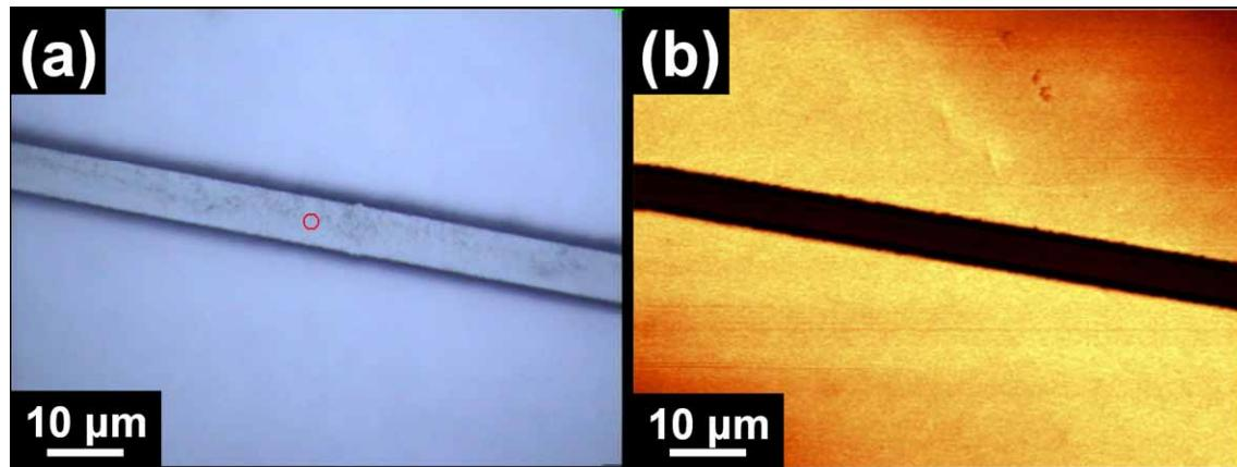
**Figure 1S** 5 micron channel waveguide fabricated from fluoroimide acrylate/SiO<sub>2</sub> nanocomposite (a) optical micrograph and (b) confocal micrograph.
