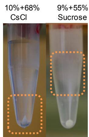
Figure S3. Digital camera images of differential centrifugation by using CsCl gradient and sucrose gradient, respectively
