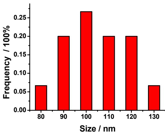
Figure S2. Size histogram of several fractions of TiO<sub>2</sub> nanospheres (TL114) separated after second-round centrifugation at 5000 rpm for 5 minutes. The calculation used about 20 particles in each fraction.
