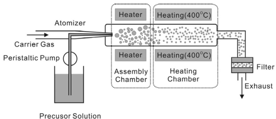
Figure S1. Schematic of the aerosol-assisted synthesis system.
