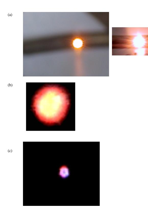
Fig. 1. NOEPLED in action (a) and beam profiles: (b) – partially filtered to reduce the intensity of the light (external SRS rings are not seen) and (c) – filtered with a "neutral dark" filter to show the central part of the beam profile.
