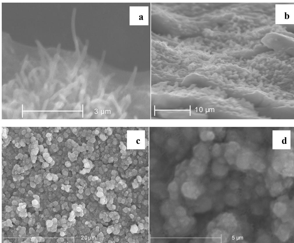
**Figure S1.** Additional ex-situ SEM micrographs of nw $\text{Fe}_2\text{O}_3$ /nt $\text{TiO}_2$  after prolonged reaction with lithium: (a,b) from iron oxide nanowires and (c,d) from iron oxide microballs onto titania nanotubes.
