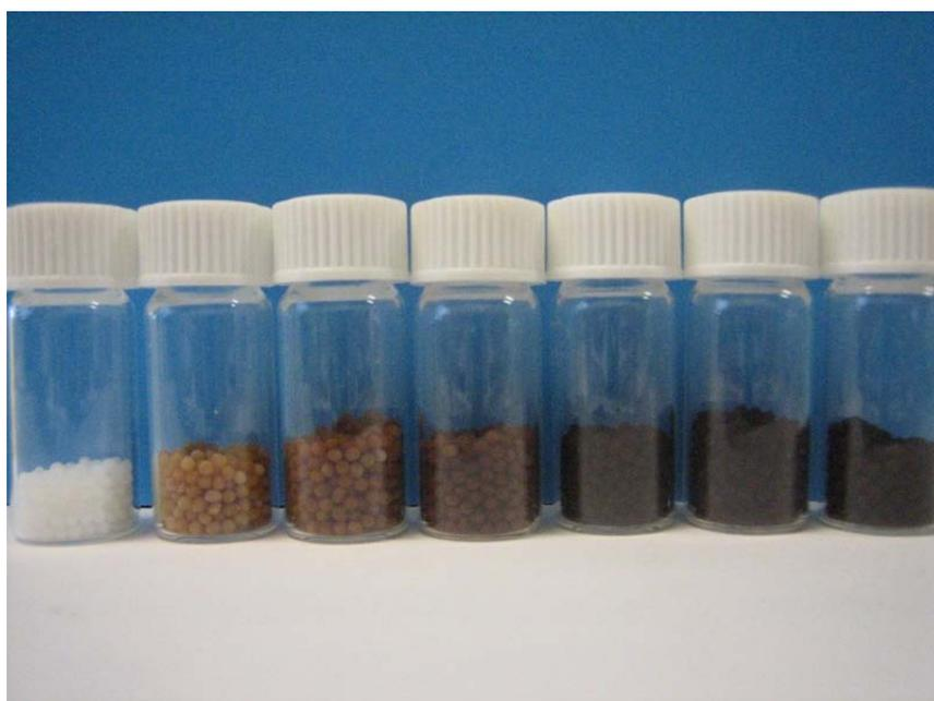
**Fig. S1:** Photograph of the MS beads series (each sample is characterized by a different value of  $\Phi_{Fe_2O_3}$ ; from left to right  $\Phi_{Fe_2O_3}$  increases from 0 to 2.1%)
