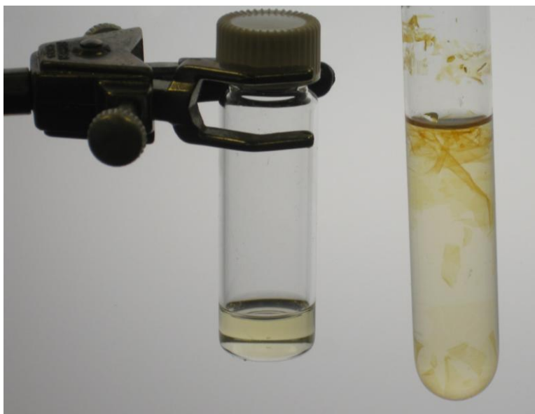
Fig. S9 Photograph of RTATT photopolymerized in chloroform for 20 h. Shown on the left is a sample without any solvent evaporation and on the right a sample with partial solvent evaporation resulting in macroscopic sheet formation.
