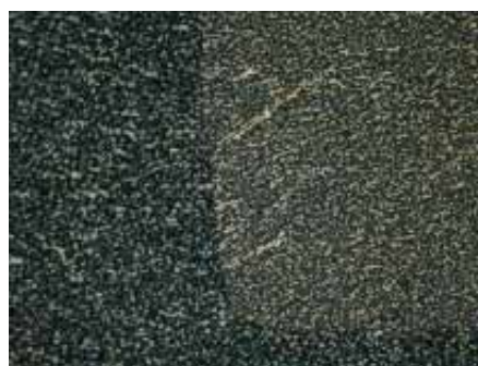
Fig. ESI 5: Textures of the crystalline phase of compound 28 /KB93/11c in a 6 \mu\text{m} cell at 162 °C. By de-crossing of one polarizer from the 90° state chiral domains become apparent: a) decrossing by + 15°; b) decrossing by -15°.
