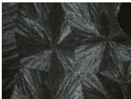
Fig. ESI 4: Texture of the crystalline phase CrIII of compound 31 /KB 70/11e at 135 °C
