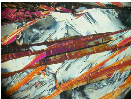
Fig. ESI 1: Microphotograph of compound 2 (2676) showing two different crystalline modifications at 146 °C on cooling: grey: CrI; brownish-orange: CrII
