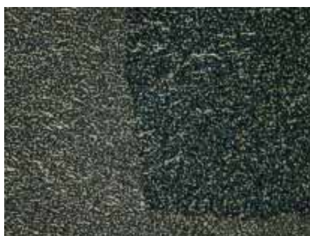
Fig. ESI 5: Textures of the crystalline phase of compound 28 /KB93/11c in a 6 \mu\text{m} cell at 162 °C. By de-crossing of one polarizer from the 90° state chiral domains become apparent: a) decrossing by + 15°; b) decrossing by -15°.
